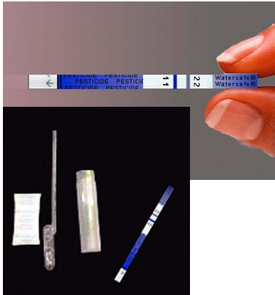
Figure 2-1. Silver Lake Research Corp. Watersafe ® Pesticide Test
