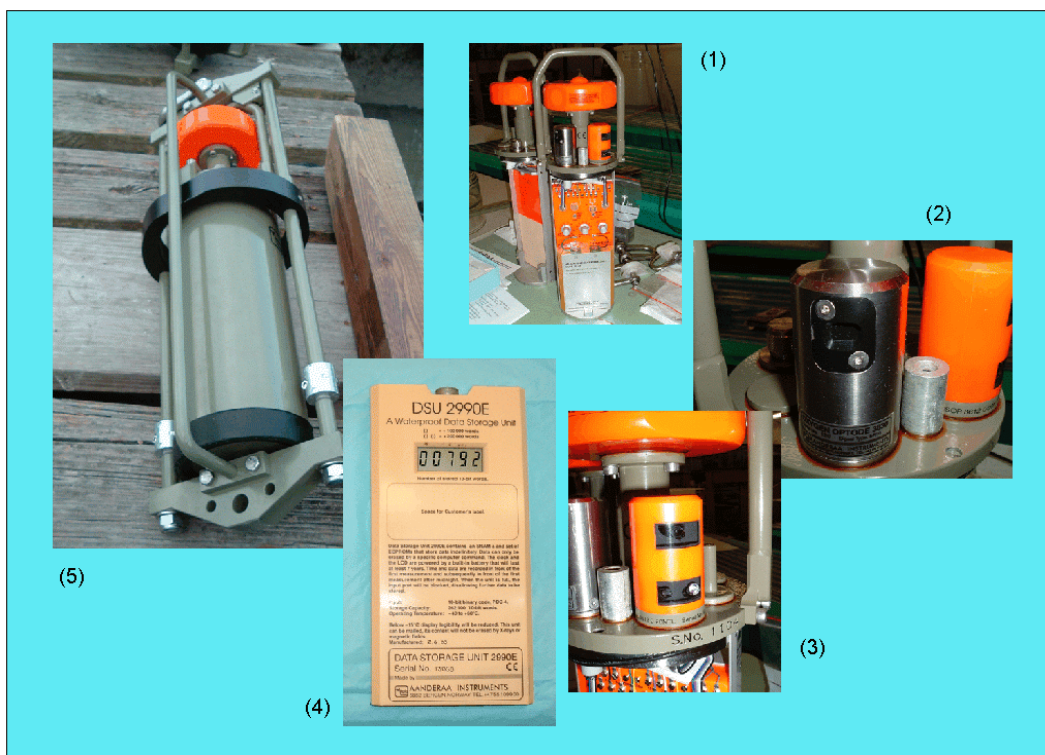
Figure 6-1. Mk II with Optode 3830 Prior to Deployment. Starting at the top center and proceeding clockwise: (1) close-up of clean Mk II with housing removed, (2) close-up of Optode 3830, (3) clean turbidity probe, (4) data storage unit, (5) Mk II dock with housing and protective side bars.
