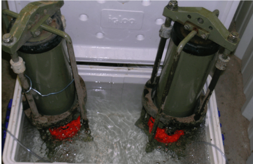
Figure 6-3. Cleaned and Reconditioned Mk II with Optode 3830 in Storage Tank Used Between Deployments
