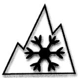
If the manufacturers choose to mark their snow tires with the Alpine Symbol, the mountain profile must have a minimum base of 15 mm and a minimum height of 15 mm, and must contain three peaks with the middle peak being the tallest. Inside the mountain profile, there must be a six-sided snowflake having a minimum height of one-half the tallest peak.
