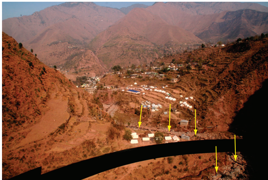
Figure 10. Aerial view of tributary stream drainage near Hattian. Location of tent camp in middle ground is on a smooth ramp just above the tributary stream (arrows) whose channel is curving to the left. This area is likely to be subject to severe runoff, or superelevation, of floodflow immediately following a potential breach of the Karli stream landslide dam.
