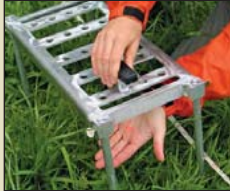
Figure 12.3 – A fixed frame can be adapted to allow for the positioning of a laser pointer at 20 points in the frame. Soil cover or plant cover attributes are recorded at each laser point. The frame in this example is 8 in by 20 in, with 2 in spacing within rows and 4 in spacing between rows. The laser is a Class IIIa red laser diode module that produces a 1mm dot.
