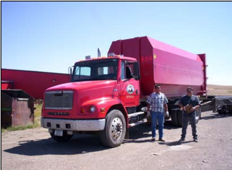
Figure 9: Truck purchased by IHS along with trailer to haul compaction containers to RCRA compliant landfill.
