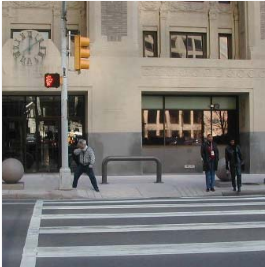
Figure 60. Intersection in Dallas’ Central Business District where longer walk and “FLASHING DON’T WALK” intervals can be put into service by depressing the push button for five or more seconds.
