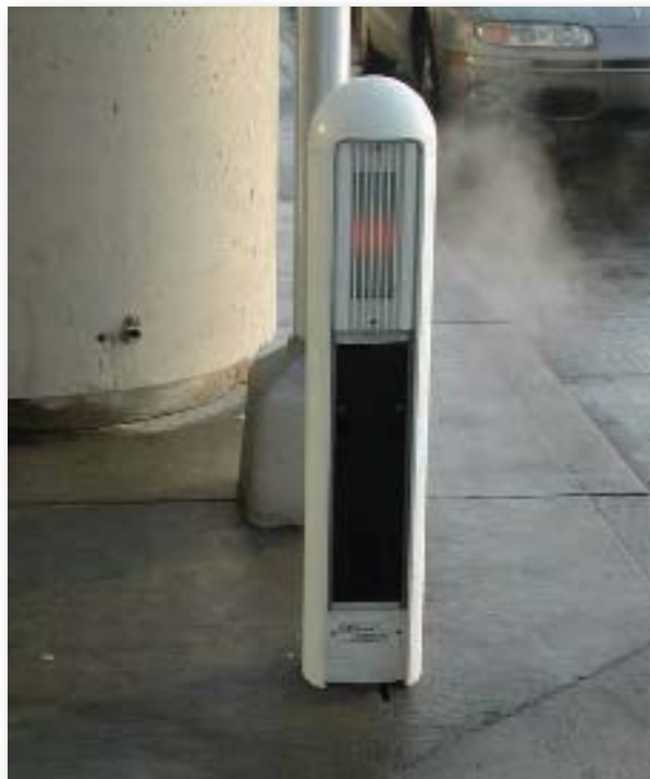
Figure 51. Pedestrian detection system that employs motion detection technology in Detroit.
