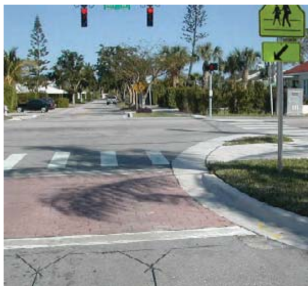
Figure 70. Photograph of same intersection in West Palm Beach showing the traffic signal heads, the loop, the brick pavement, the transverse crosswalk markings and the school crossing sign.
