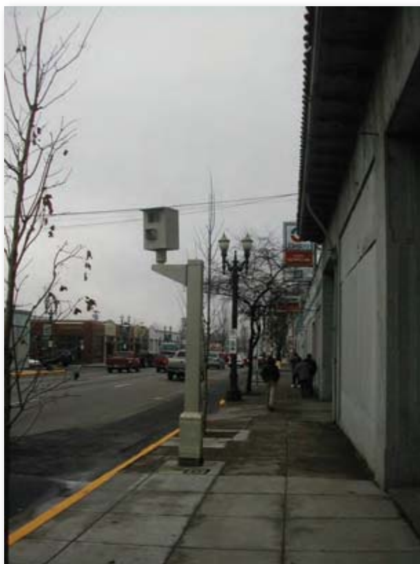
Figure 101. View of camera for a red light running automated enforcement system.
