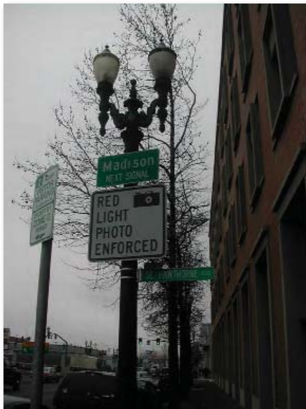
Figure 100. View of advance sign for a red light running automated enforcement system in Portland.
