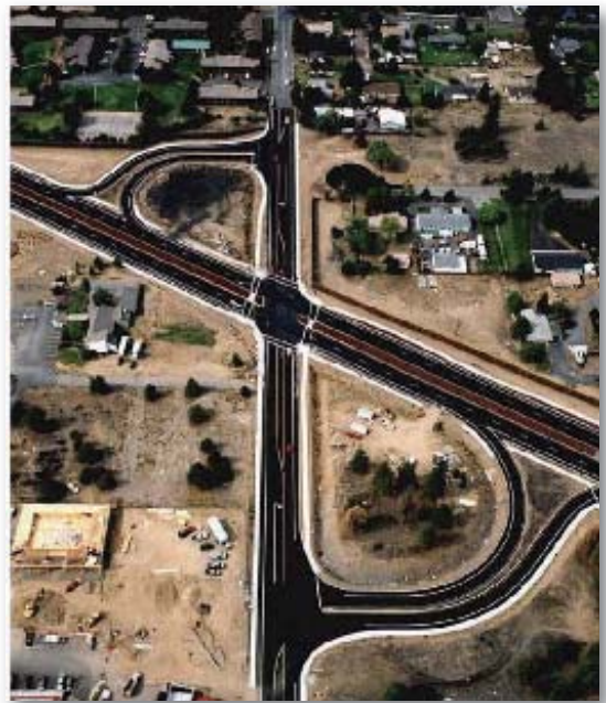
Figure 84. At-grade intersection with jug-handle ramps in two quadrants located in Bend, Oregon.
