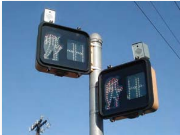
Figure 44. Audible pedestrian signal heads and speakers in Charlotte.
