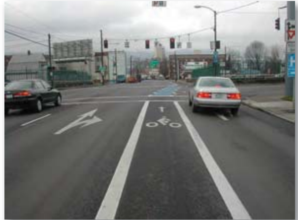
Figure 36. Example of a blue bike lane between a dedicated right turn lane and a shared use right-and-through lane in Portland.
