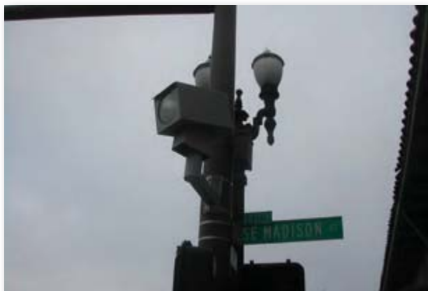
Figure 102. View of strobe light at the intersection for a red light running automated enforcement system in Portland.
