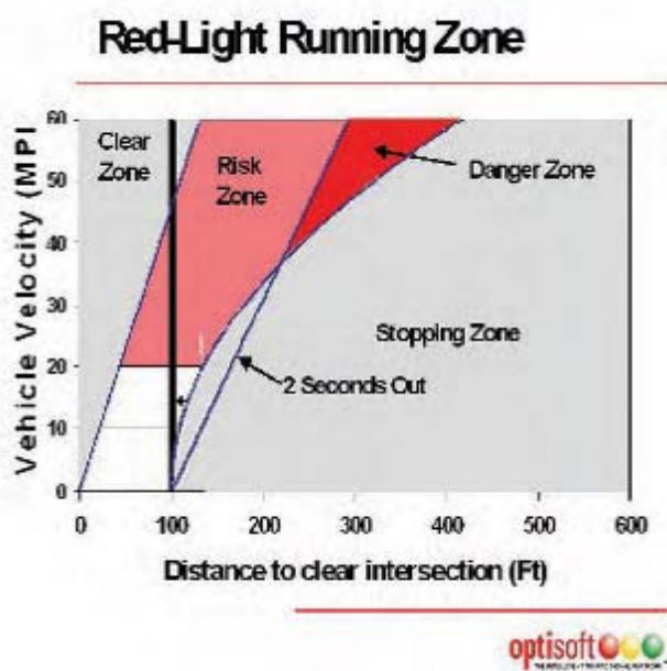
◀ Figure 62. Speed prediction algorithm for Richardson experimental red clearance interval hold. (Courtesy of the City of Richardson).
