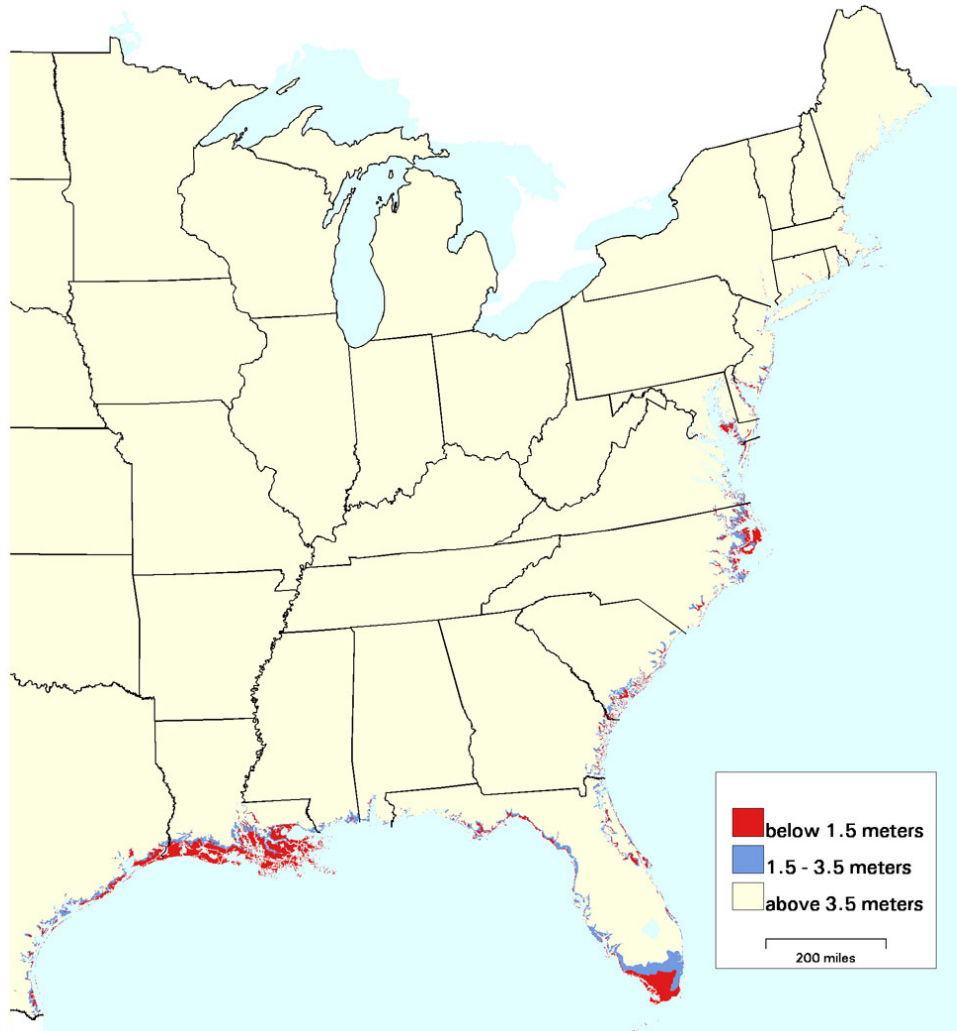
Figure 2. Map of lands close to sea level along the U.S. Atlantic and Gulf Coasts. Although the results nominally are in meters, the 1.5 meter contour is primarily based on the 5-ft NGVD contour from USGS topographic maps. Source: Titus and Richman (2001). 6
