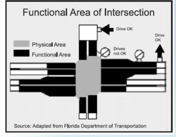
Driveways should not be located within the functional area of an intersection.
