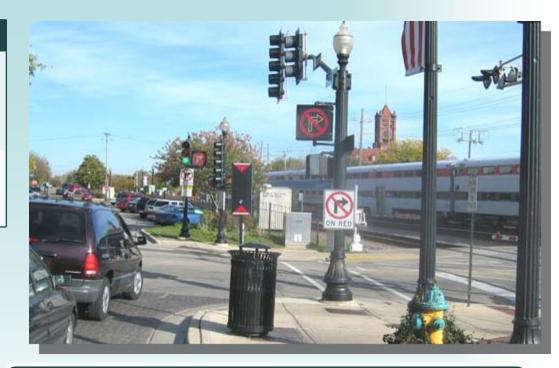
When the right-of-way needed to provide [left-turn] storage is not available, left-turn restriction is a means of eliminating [safety and operational] problems.
