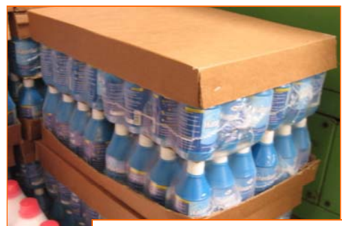
PSI/Kenya packaging to prevent breakage (eight groups of 12 packaged in boxes, later shrink-wrapped)
