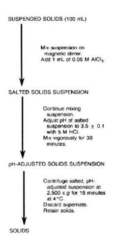
Figure 2. Flow Diagram of Method for Elution of Virus from Solids
