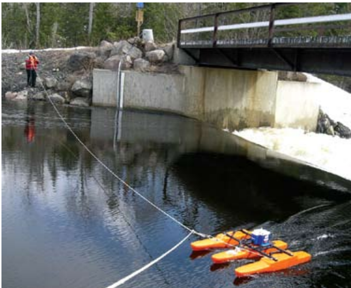
Elizabeth Nystrom of USGS uses an Acoustic Doppler Current Profiler to measure discharge in Fishing Brook at County Line Flow.
