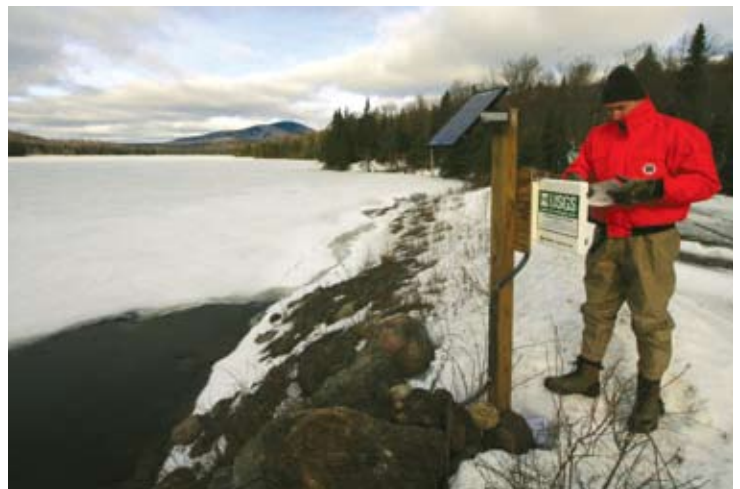
Jakob Schelker downloads data from the USGS stream gage that records the discharge of Fishing Brook at County Line Flow.
