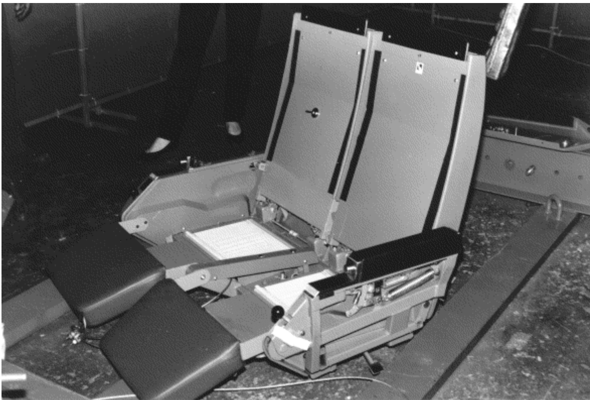
Figure 3-1. Photograph of Frame of Amtrak's Traditional Seat Pair
