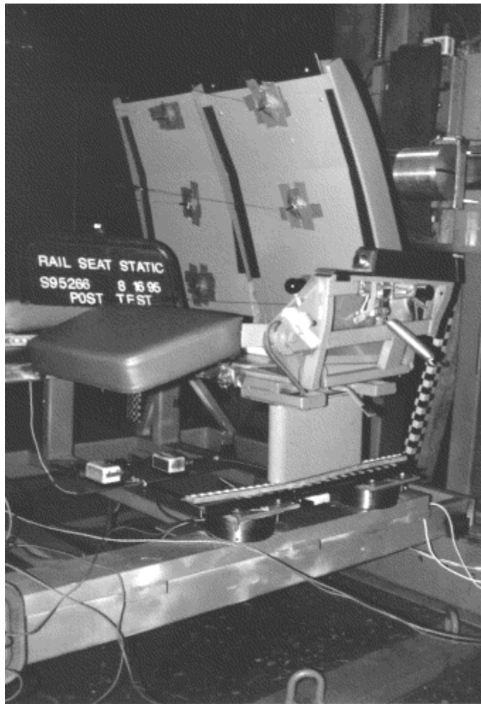
Figure 5-2. Head-Load Quasi-Static Test, Seat Pair Post-test Condition
