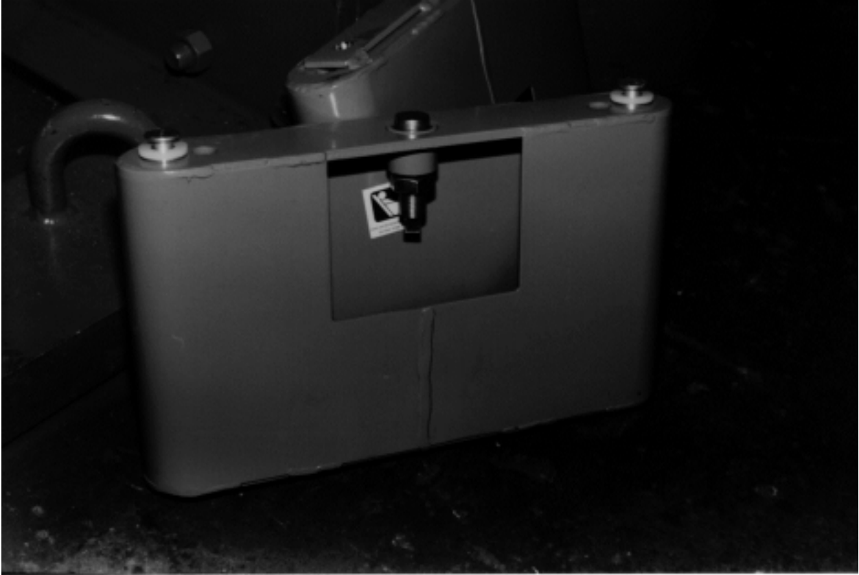
Figure B-4. Floor Pedestal Photograph Showing Access Cutout for Locating/Locking Pin and Bottom Plate
