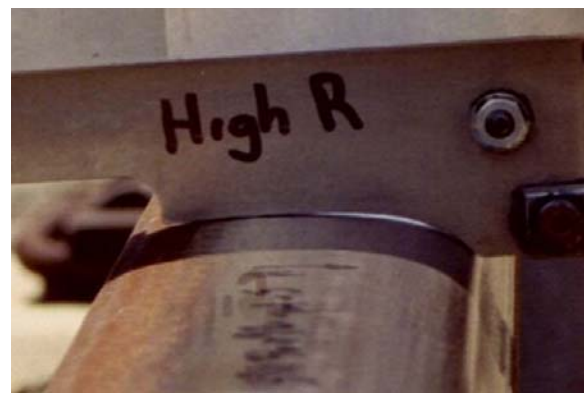
Figure 5. Even with significant gauge side contact, the 2001 Amtrak high-rail template suggests that the gauge side needs to be raised even higher. This would lead to severe 1-point contact and likely problems of rail fatigue.
