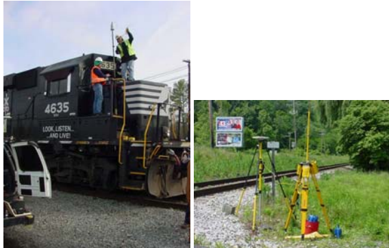
Figure 5. Left: GPS antenna being adapted to a locomotive. Right: Temporary GPS base station needed to achieve centimeter precision from the roving GPS unit.
