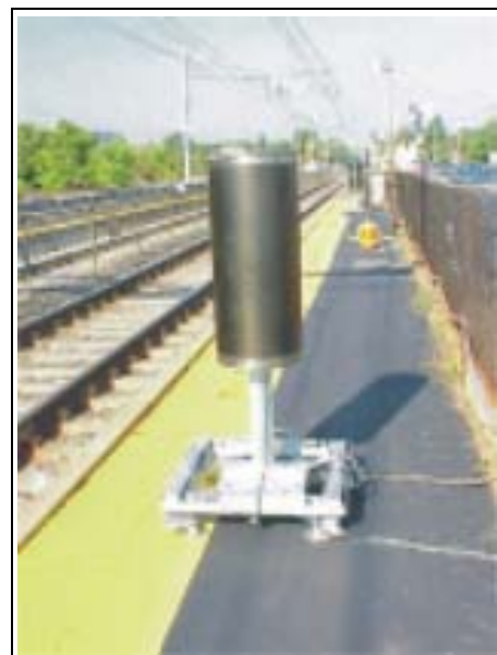
Figure 16. Cylindrical Instrumented Dummy for Measuring Force from Aerodynamic Interaction with a Passing Train
