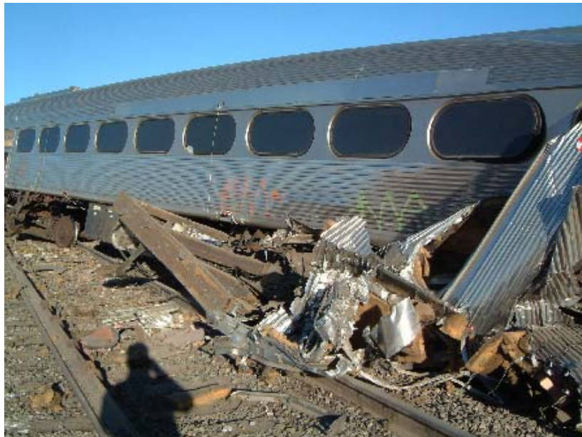
Figure 6. End Frame is Lying Face Down Over the Left Rail, Oriented Approximately 90° with Respect to the Track
