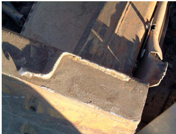
Figure 14. Location at which Roof Rail Was Connected to Left, Rear Side of Antitelescoping Plate
