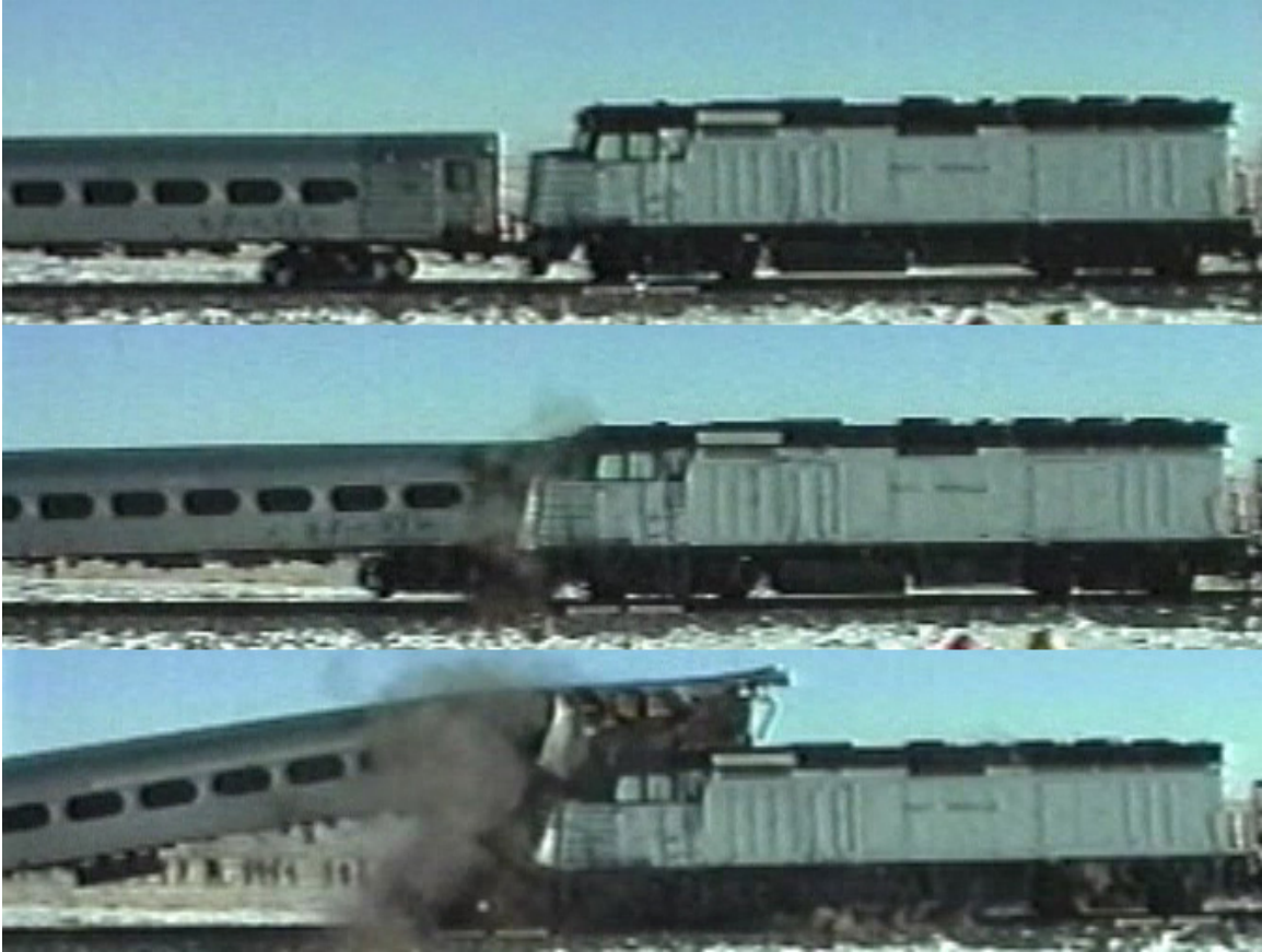
Figure 2. Images Taken from High-Speed Film Showing the Cab Car Overriding the Standing Locomotive
