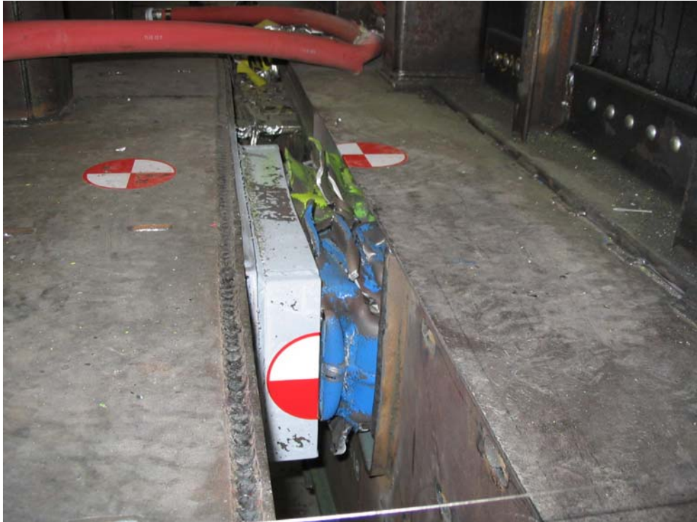
Figure 11. Condition of the Primary Energy Absorbers After the One-Car CEM Test; End 248A
