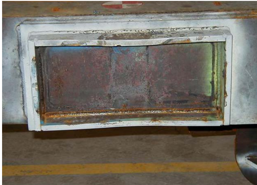
Figure 8. Back Surface of the End Beam After the CEM Test in the Area at Which the Primary Energy Absorber Contacts
