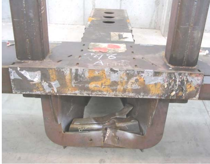
Figure 6. Bell Mouth on End 248A After the One-Car CEM Test
