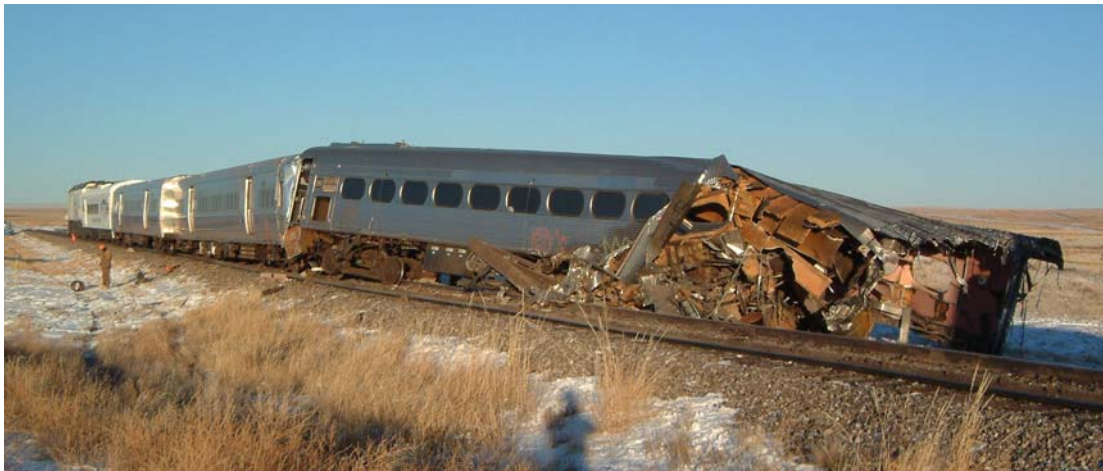
Figure 1. Cab Car Crush in the Train-to-Train Test
