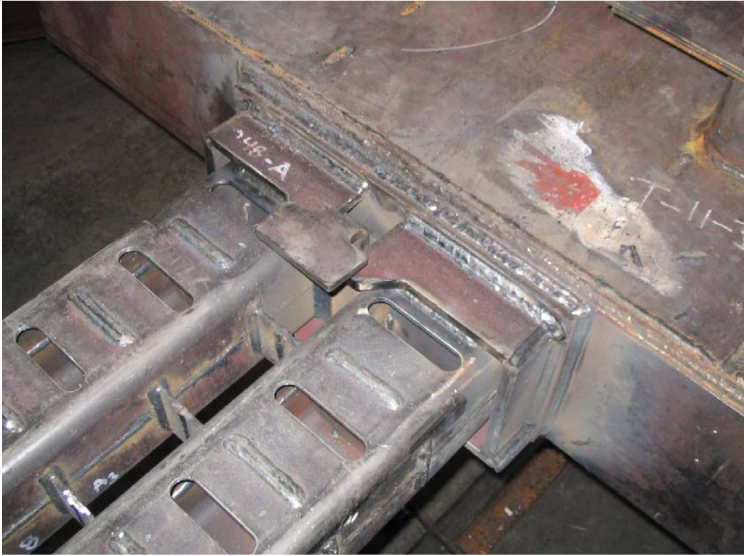
Figure 18. Modified Inboard Surface of the End Beam in the Vicinity of the Primary Energy Absorbers and the New Retention Device
