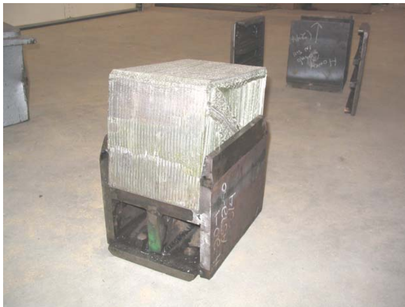
Figure 4. Push-Back Coupler Honeycomb Absorber with Its Support Element After the Full-Scale Test
