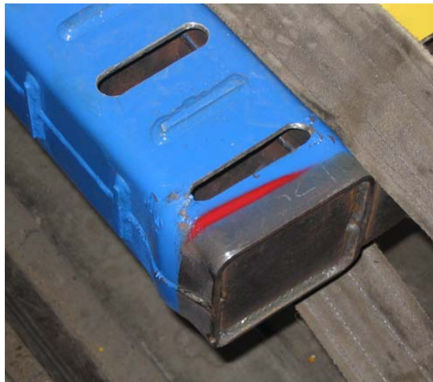
Figure 12. Primary Energy Absorber from Car End 248B After the Two-Car Test
