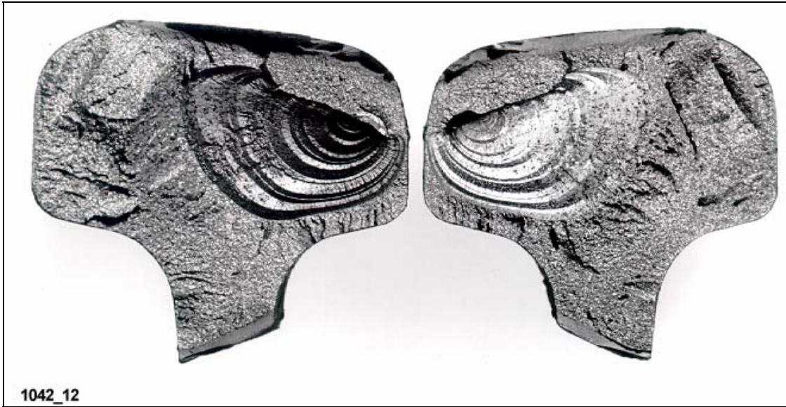
Figure 1. Detail Fracture in the Head of a Rail
