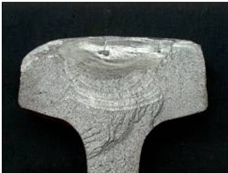
Figure 5. Welded Burn Fracture in the Head of a Rail
