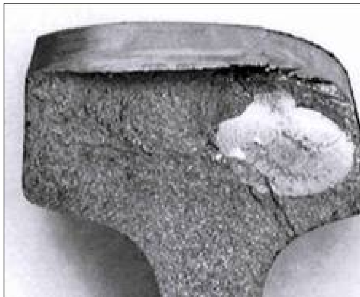
Figure 2. Compound Fissure in the Head of a Rail
