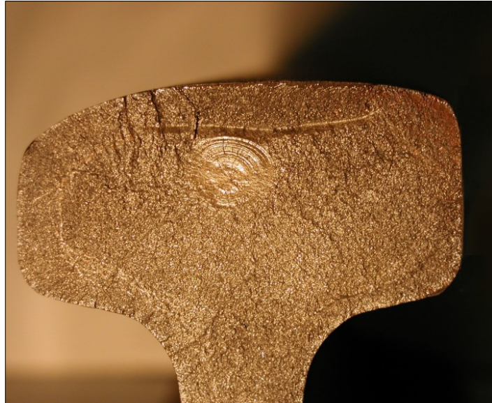
Figure 3. Transverse Fissure in the Head of a Rail
