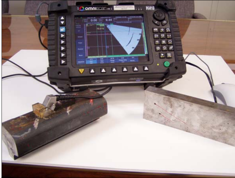
Figure 34. Omni-Scan PA System Used at FAST
