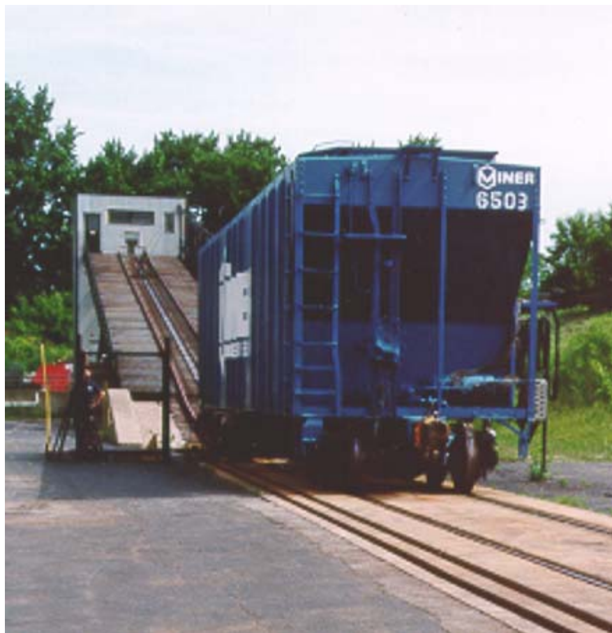
Figure 7. Hammer car on impact ramp
