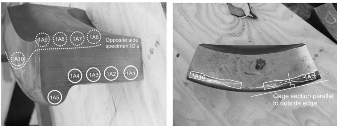
Figure 4. Schematic Layout for the Fatigue Specimens in Each Wheel Section
