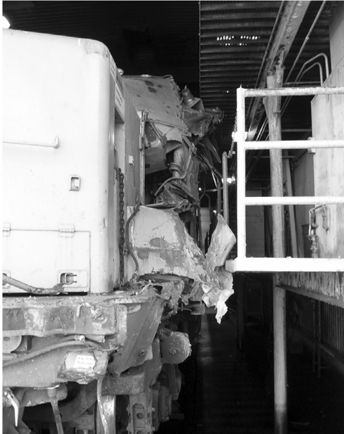
Figure 36. RCL3 view of damaged sheared left side of lead RCL
