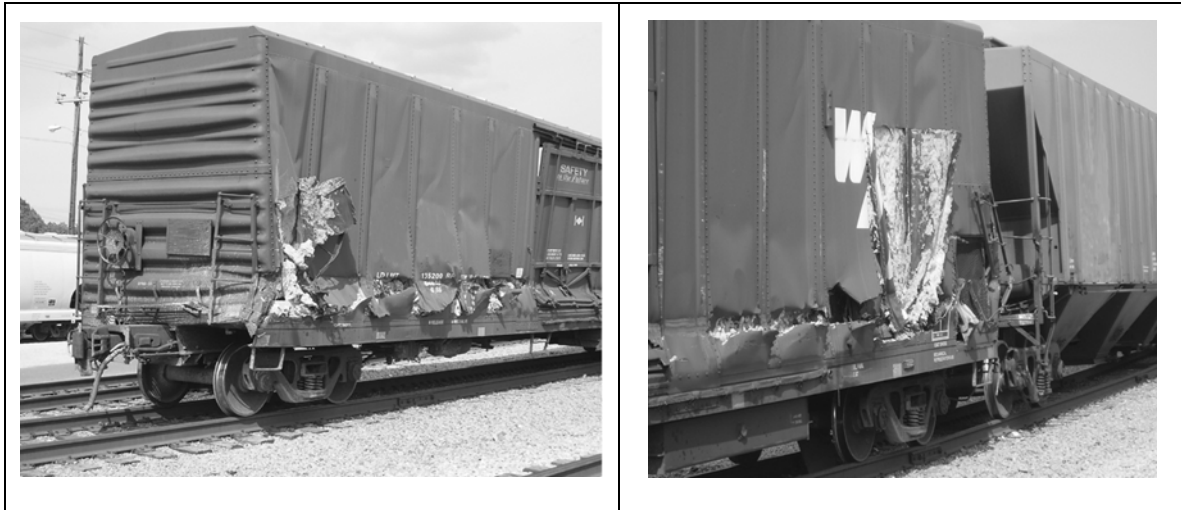
Figure 17. RCL1 damage to box car
