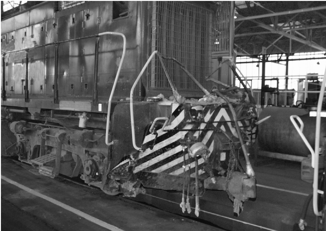
Figure 67. RCL6 damage to trailing locomotive
