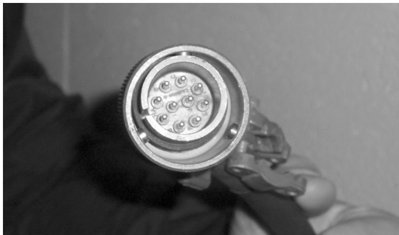
Figure 70. RCL6 view of antenna cable pins and connector
