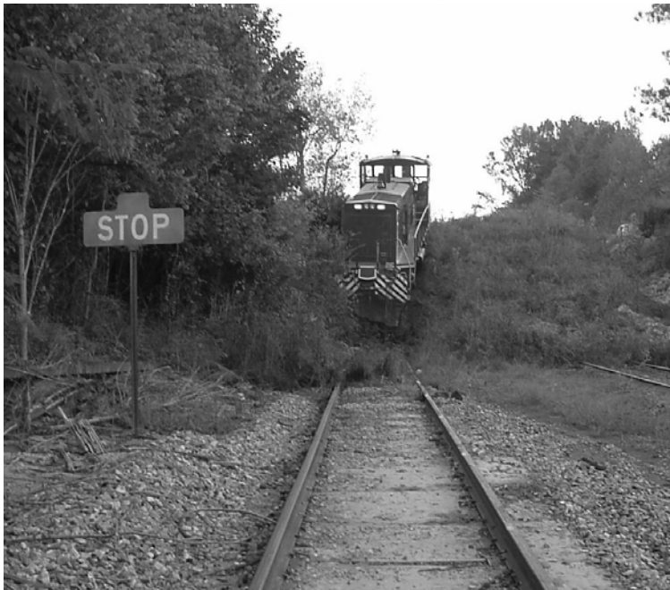
Figure 66. RCL6 view of lead (RCL) locomotive derailed up embankment (modified and reprinted with permission of the railroad)
