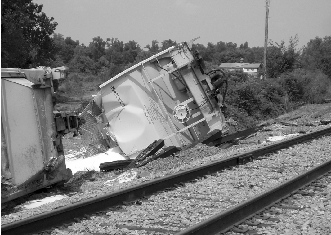
Figure 34. RCL3 derailed hopper car of inbound road train
