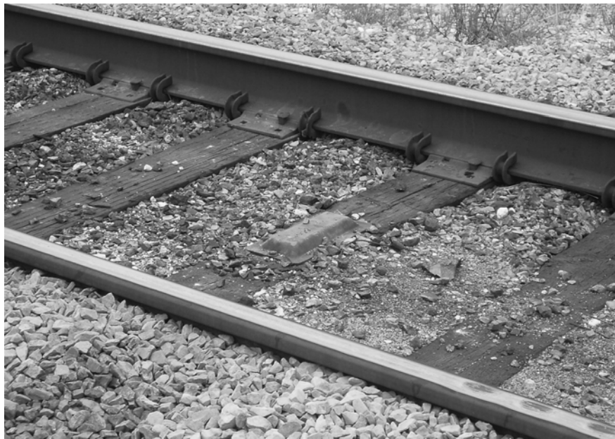
Figure 50. RCL5 passive track transponder
