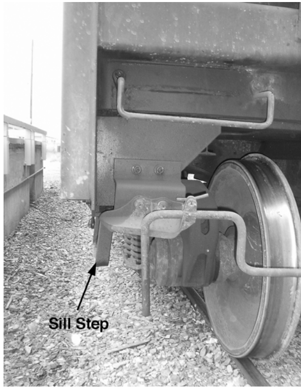
Figure 44. RCL4 side view of recessed sill step
