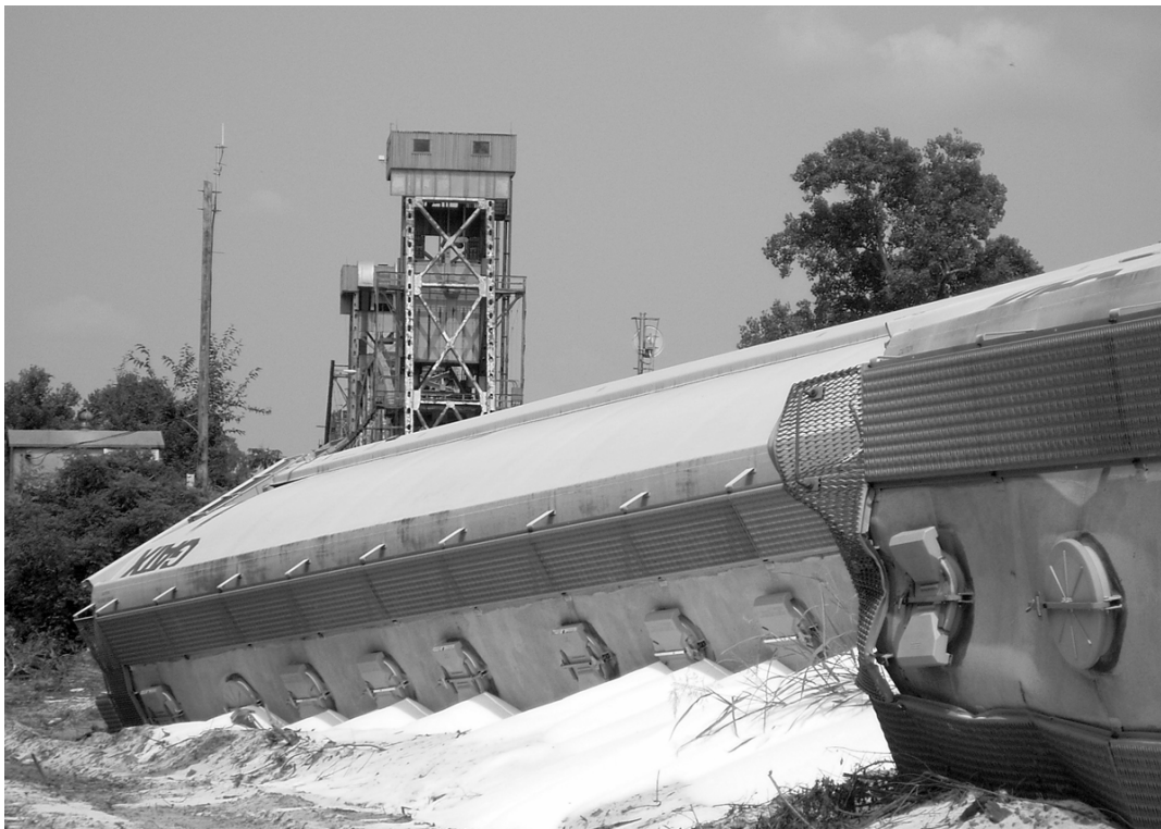
Figure 35. RCL3 spilled plastic pellets from derailed hopper car
