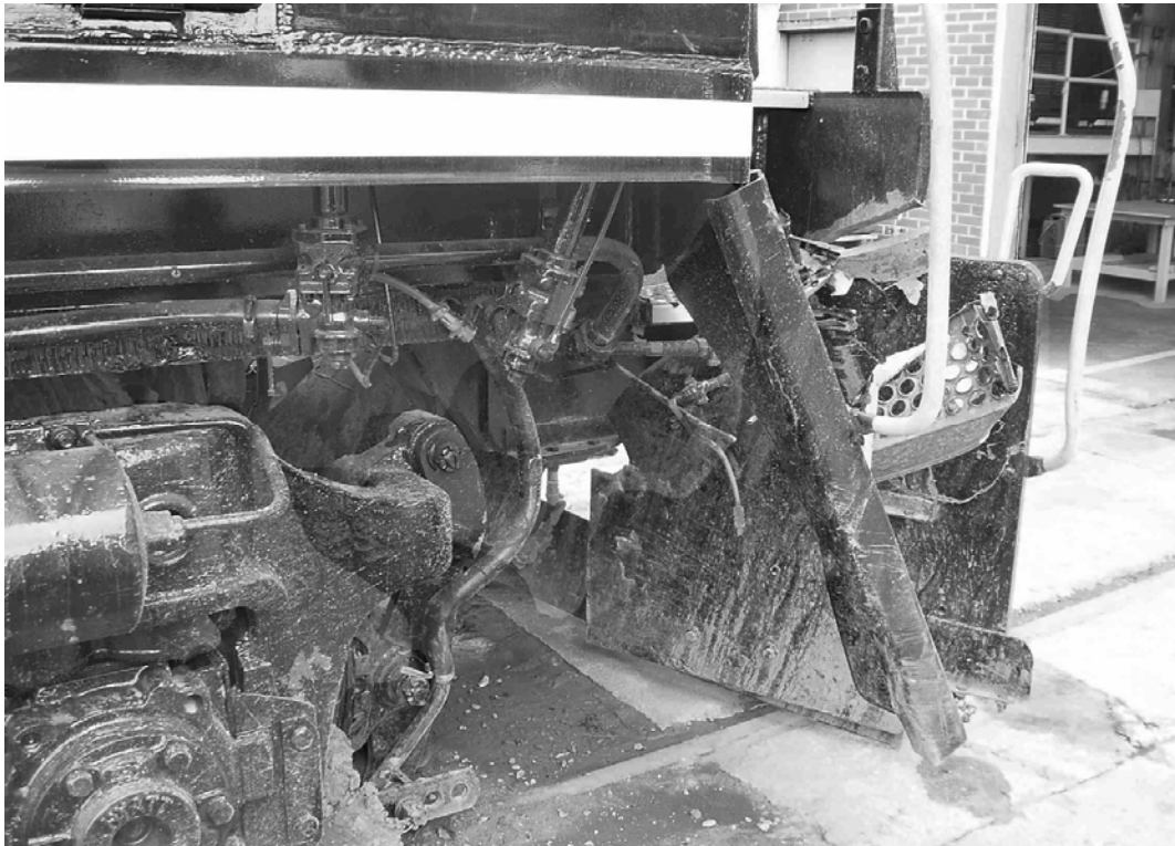
Figure 68. RCL6 damage to leading RCL
