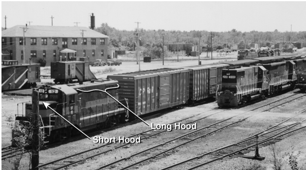
Figure 25. RCL2 example of short and long hood of locomotive
