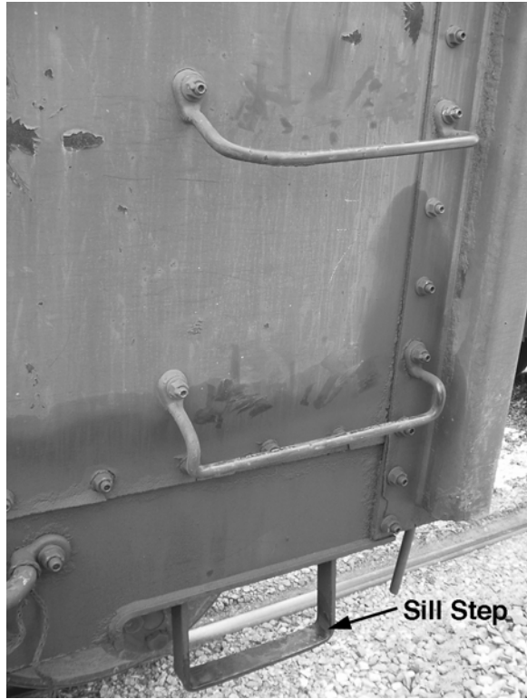
Figure 43. RCL4 front view of recessed sill step
