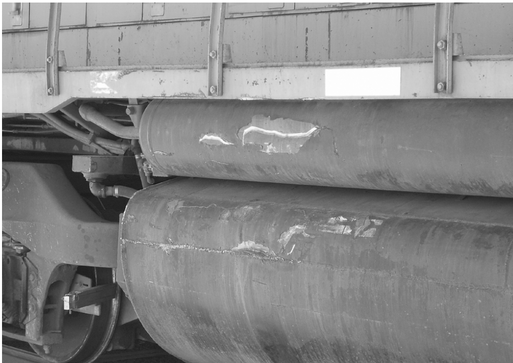
Figure 20. RCL2 damaged locomotive fuel tank
