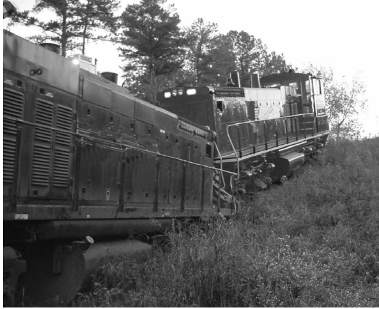
Figure 65. RCL6 view of locomotives derailed up embankment at end of track (modified and reprinted with permission of the railroad)
