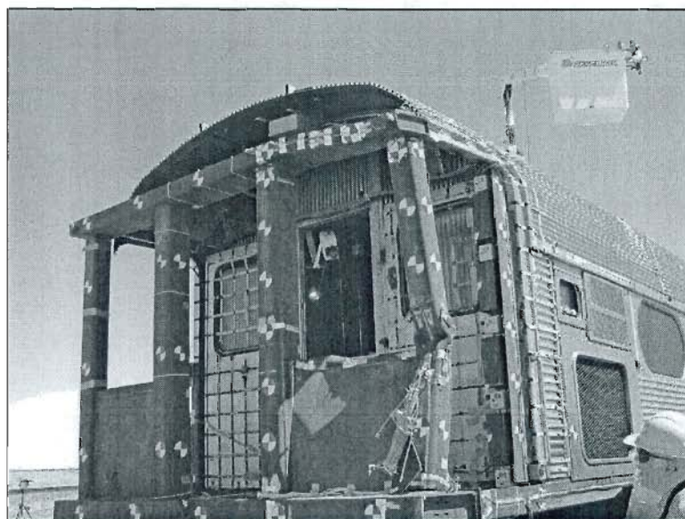
Figure 10. SOA Design Cab Car After Impact With Steel Coil
