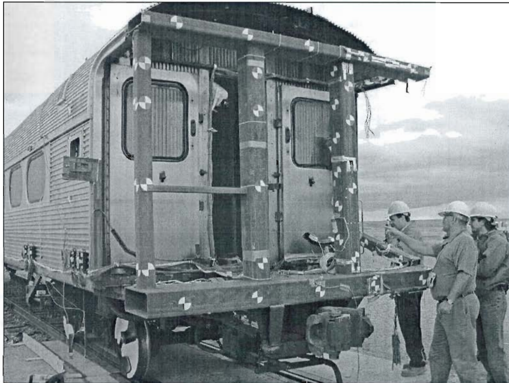
Figure 8. 1990's Design Cab Car After Impact With Steel Coil
