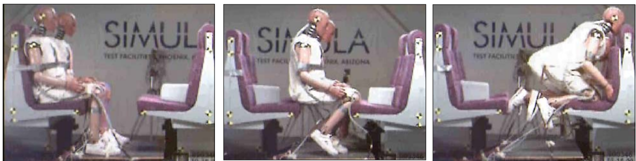
Figure 17. Test No. 1, Occupant Kinematic Sequence for Two 50th-percentile ATDs, 8 G Peak, No Table
