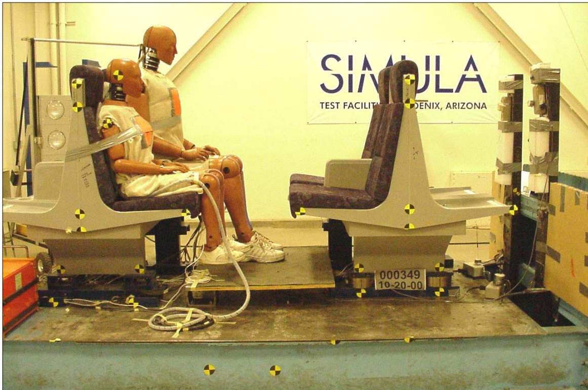
Figure 26. Pre-test Photo of Test No. 4, Baseline with 5th- and 95th-Percentile Size ATDs
