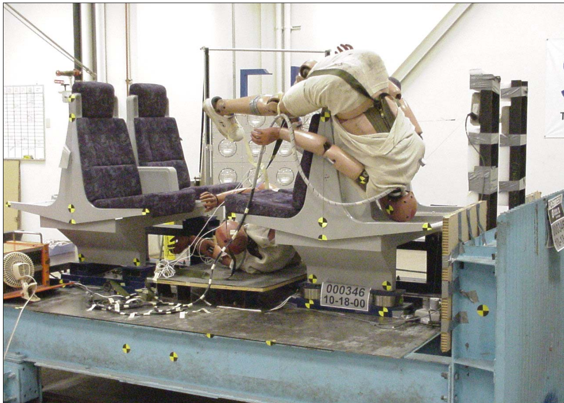
Figure 18. Post-test Photo of Test No. 1, Baseline Test
