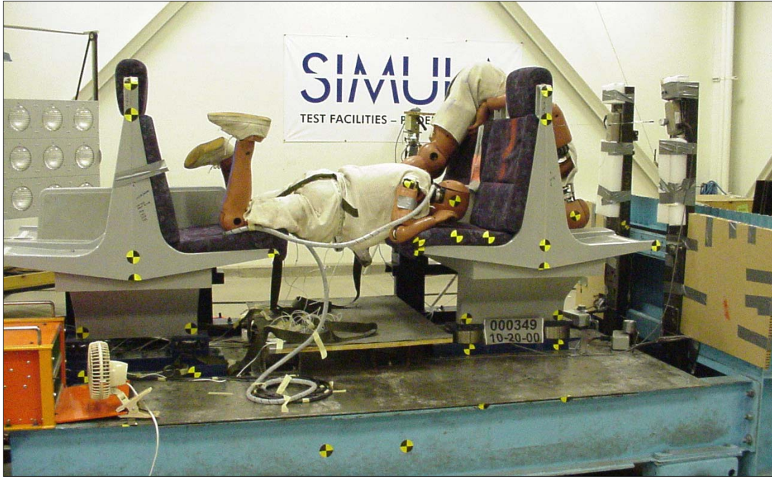
Figure 28. Post-test Photo of Test No. 4, Baseline Test with 5th- and 95th-Percentile ATDs
