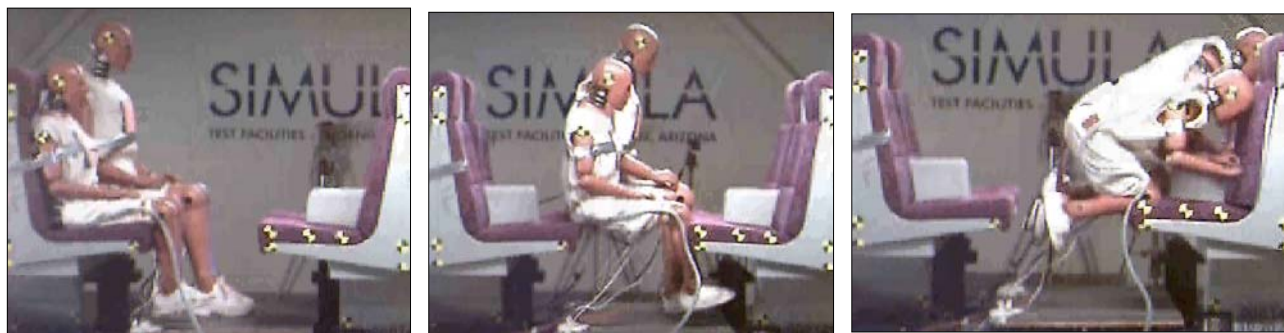
Figure 27. Test No. 4, Occupant Kinematic Sequence for the 5th- and 95th-Percentile ATDs, 8 G Peak Acceleration
