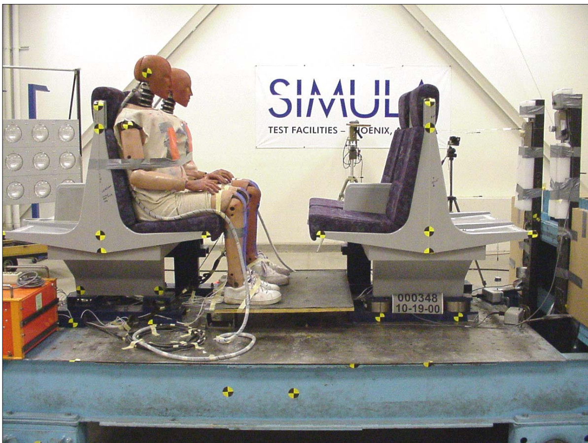
Figure 9. Dynamic Sled Test Configuration of Two Back-to-Back Facing Seats with 65-inch Seat Pitch, No Table
