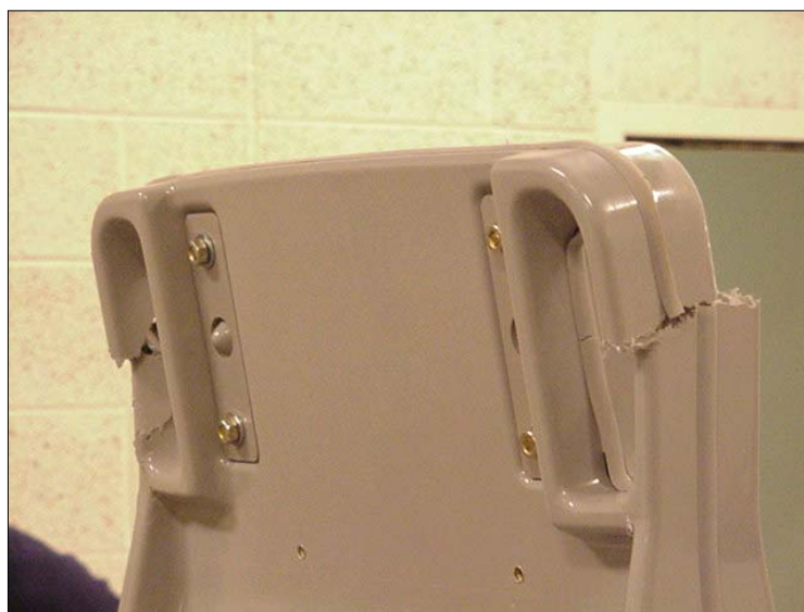
Figure 30. Broken Grab Handles
