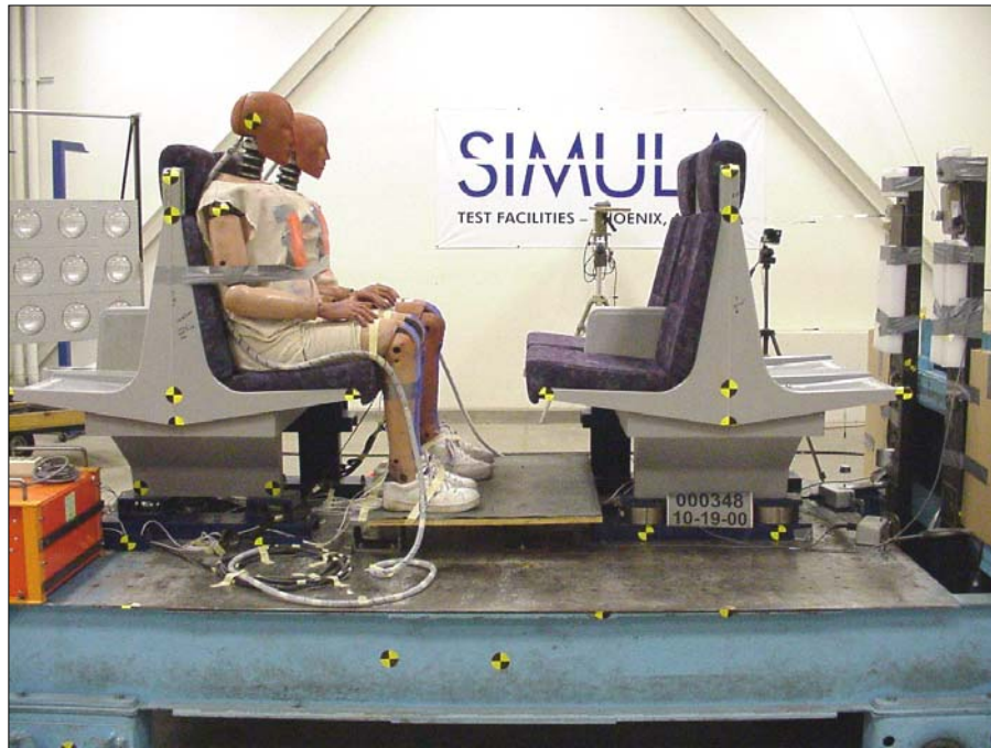
Figure 3. Bombardier Back-to-Back Opposing-Facing Seats Mounted on Simula's Dynamic Test Sled
