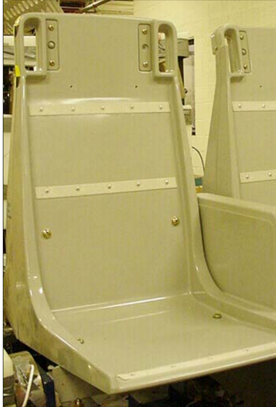
Figure 2. Thermoplastic Seat Pan/Back Structure
