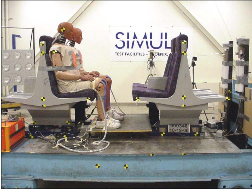
Figure 23. Pre-test Photo of Test No. 3, Baseline Configuration with 9 G Peak Acceleration
