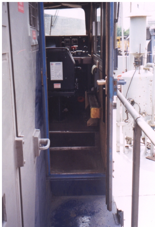
Figure 18. GE CW40-8 - door behind engineer's seat to exterior walkway
