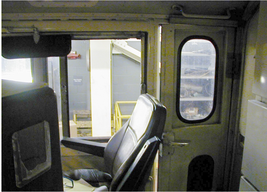
Figure 66. Cab view of side window and door for F40-PH locomotive
