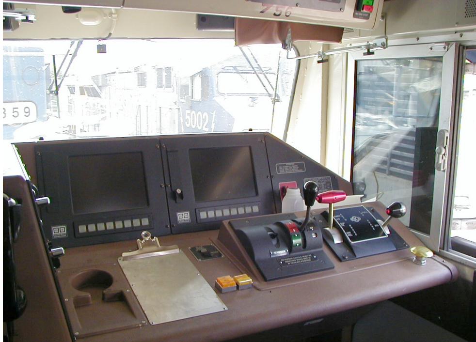
Figure 101. Desk-type station control stand
