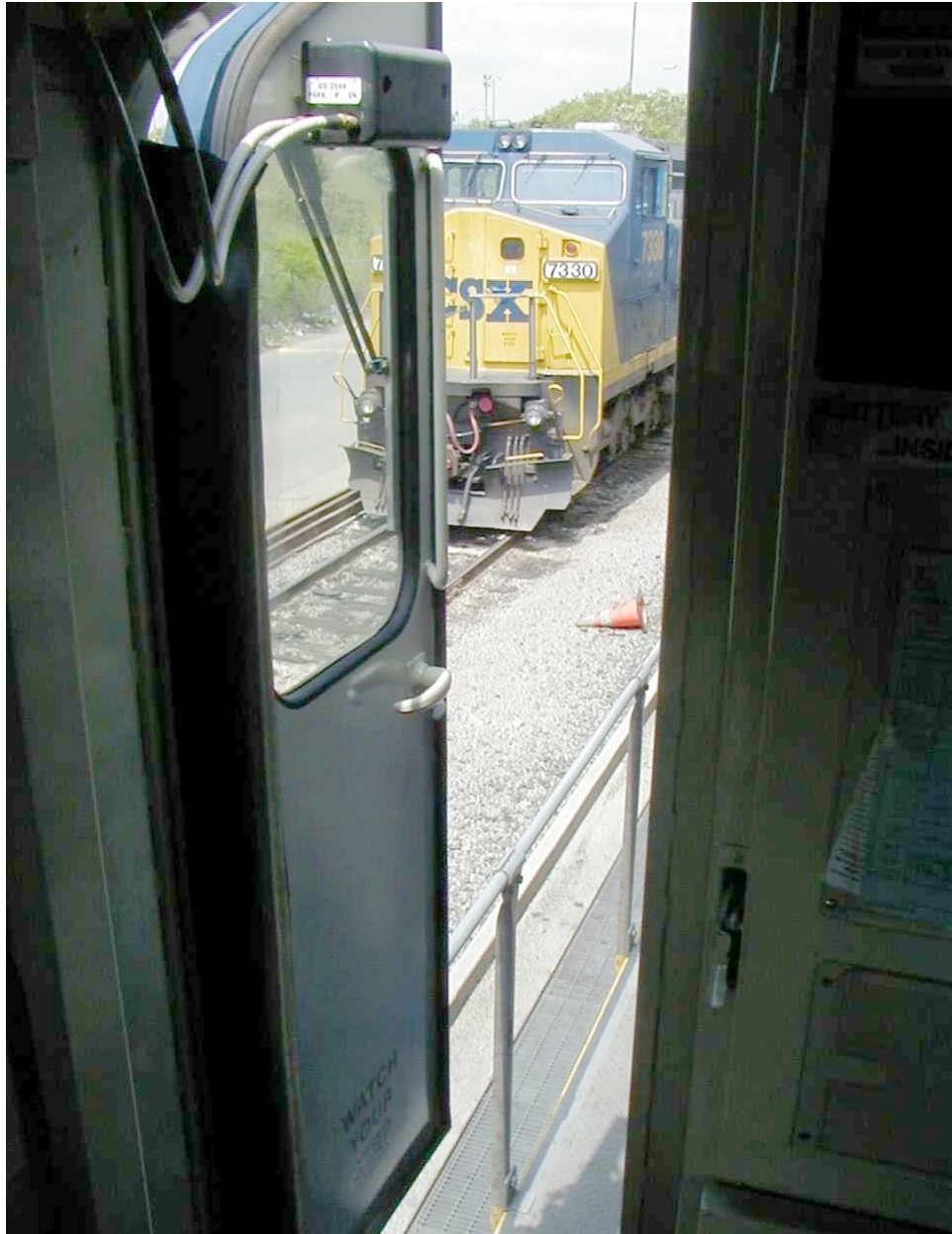
Figure 74. Rear cab door of SD-70 MAC freight locomotive
