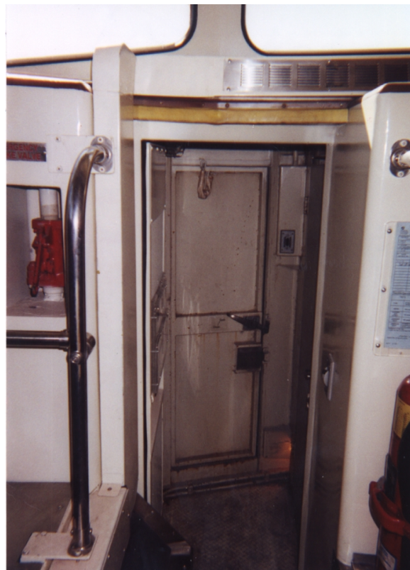
Figure 92. Narrow passageway to nose door of F59 is easily obstructed
