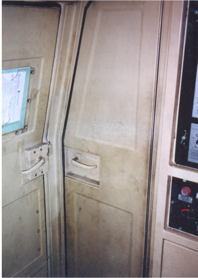
Figure 12. Side cab entry/exit door on left of photo: handle on right side of door, pull open into cab. Engine room door on right: handle (recessed) on left side of door, push to open into engine room
