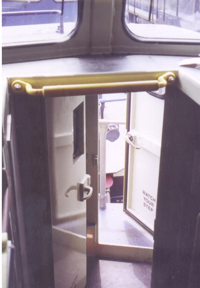
Figure 85. View from locomotive cab of SD-70 MAC to nose door (door sill 3 to 4 inches high)
