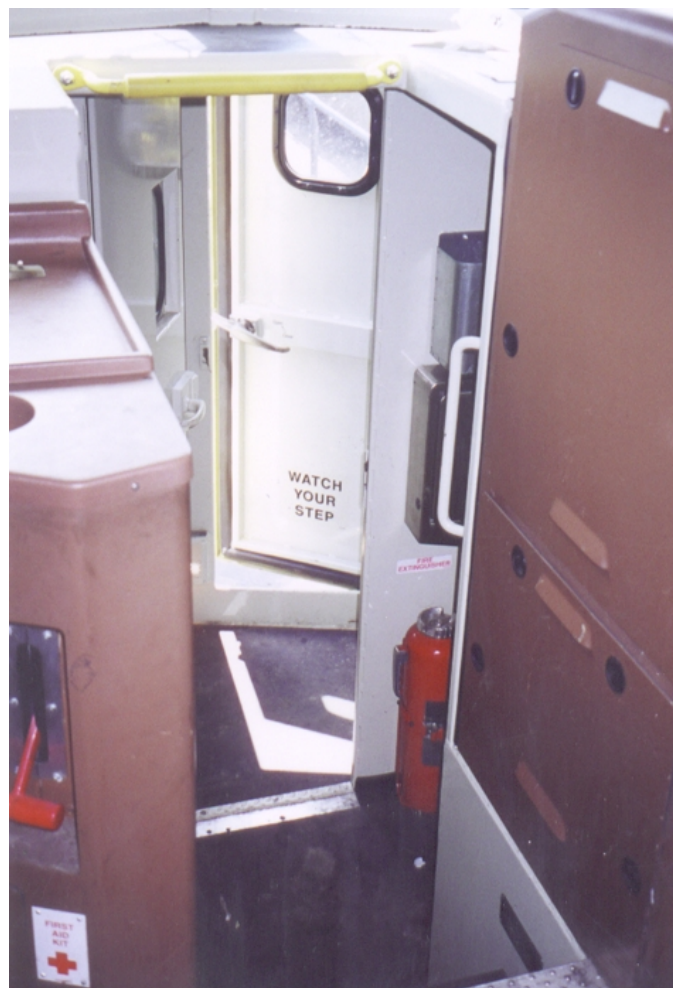
Figure 103. SD-70 MAC fire extinguisher located on cab side wall near the observer's station
