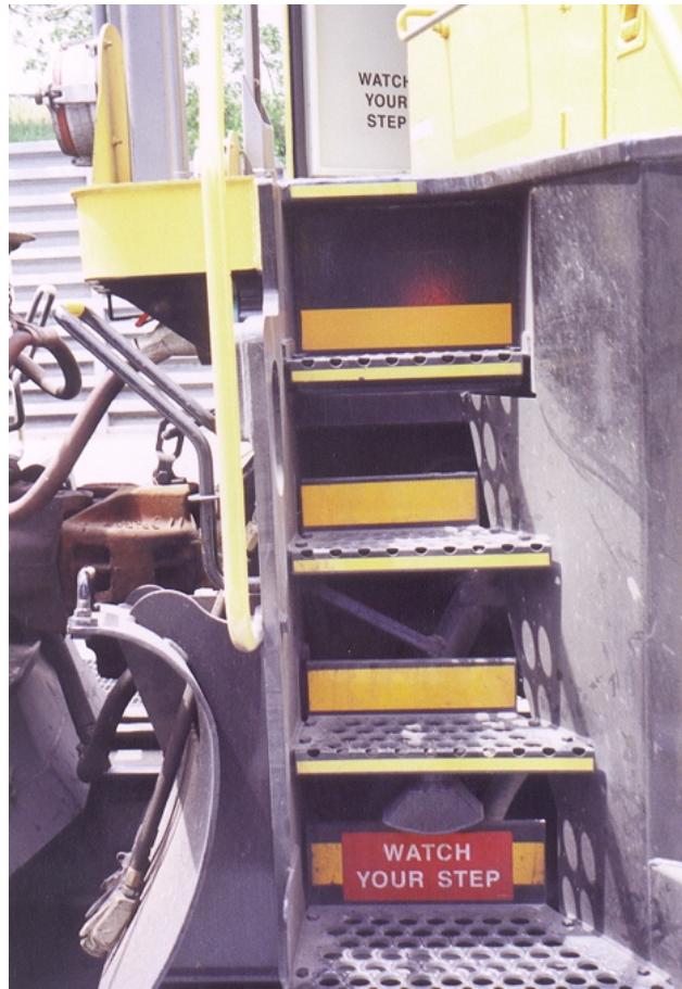
Figure 83. SD-70 MAC retroreflective step markings
