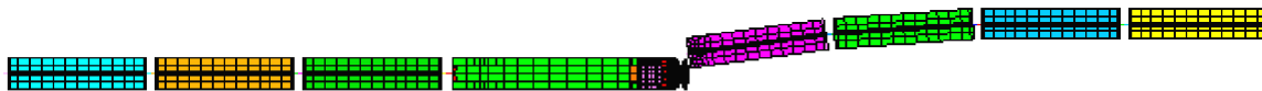
Figure 40. Top view showing a typical collision between a locomotive and hopper car consist
