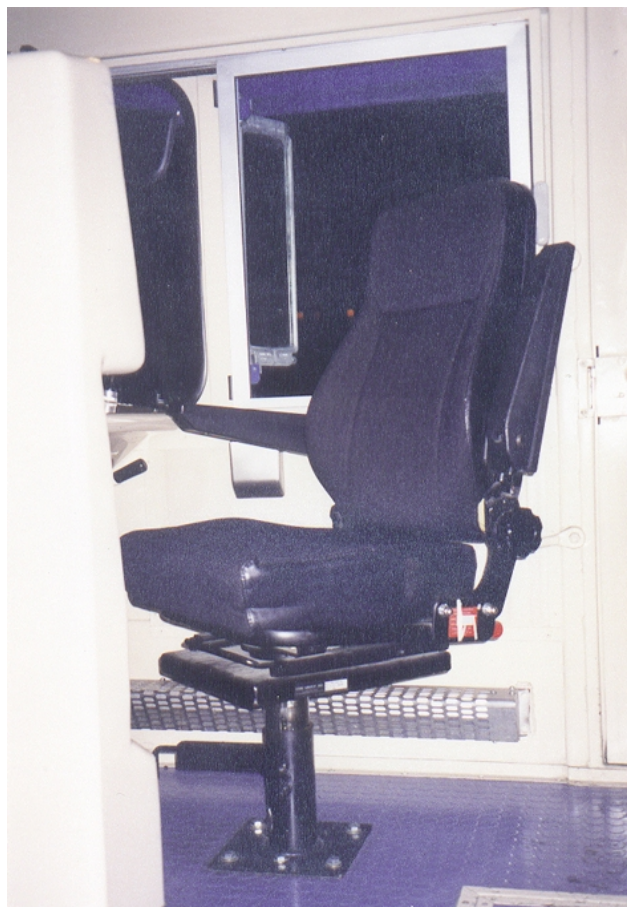
Figure 1. Cab seat mounting - F59 rebuild
