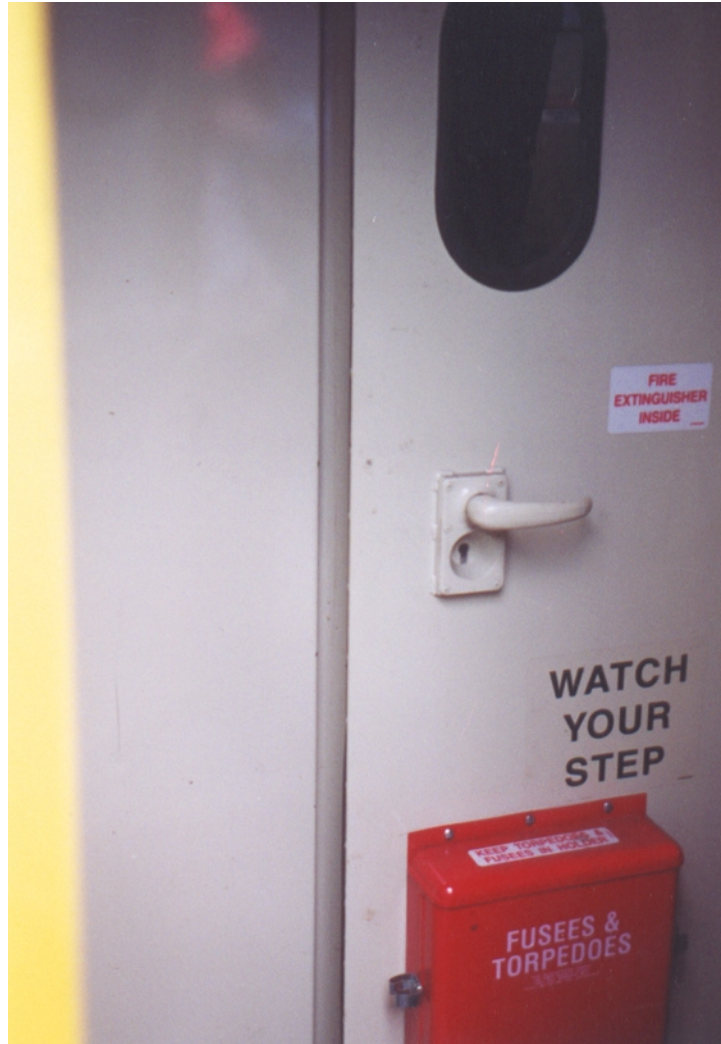
Figure 105. SD-70 MAC fuses and torpedoes box mounted on the nose side of the vestibule door
