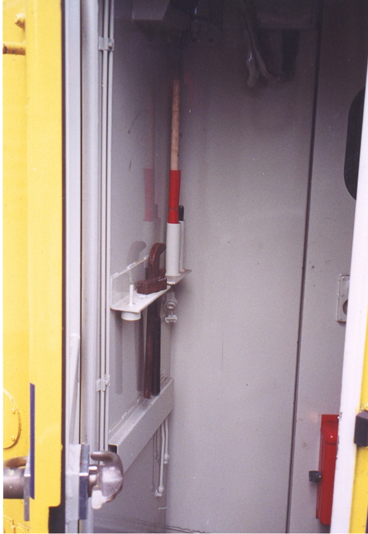
Figure 106. SD-70 MAC emergency tools located in the nose side of the vestibule
