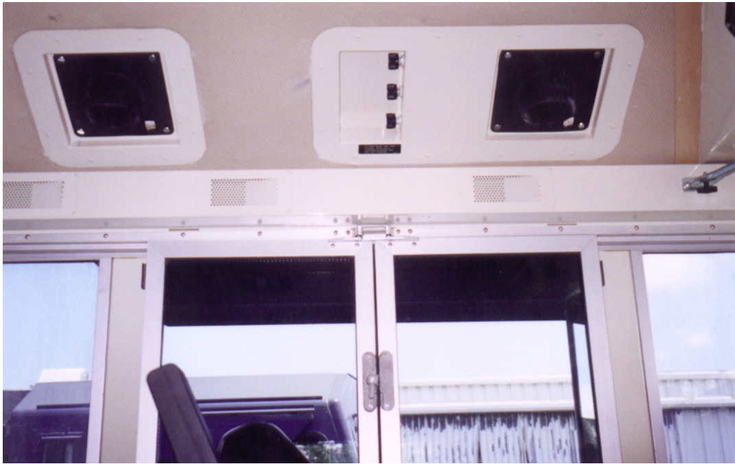
Figure 91. Overhead cab lighting, over the seat opposite engineer's seat (SD-70 MAC) (Note double-opening window)
