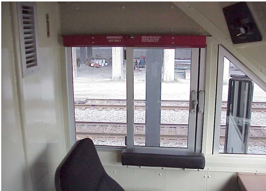
Figure 76. Interior view of F59 cab emergency exit window
