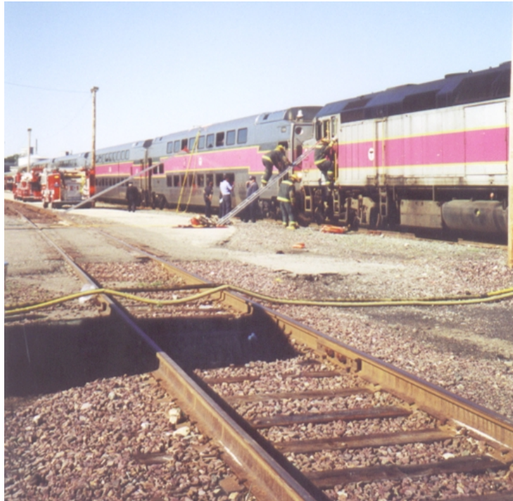
Figure 84a. Emergency responders ascending ladder and locomotive ladder to begin removal of "injured" engineer from F40 passenger locomotive
