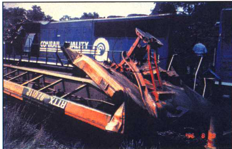
Damaged Trailer Car after Collision
