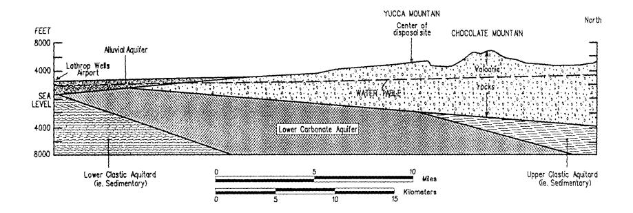
Figure ES.5-1. Schematic North/South Cross-Sectional Illustration of Thinning of Volcanic Units Beneath the Amargosa Desert [U.S. Geological Survey, *Structure of Pre-Cenozoic Rocks in the Vicinity of Yucca Mountain, Nye County, Nevada,* USGS Survey Bulletin 1647, 1985]
