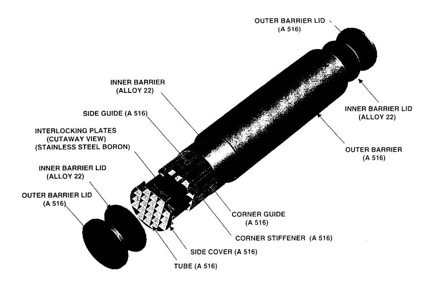
Figure ES.5-3. Waste Package for 21 PWR Uncanistered Fuel Assemblies
