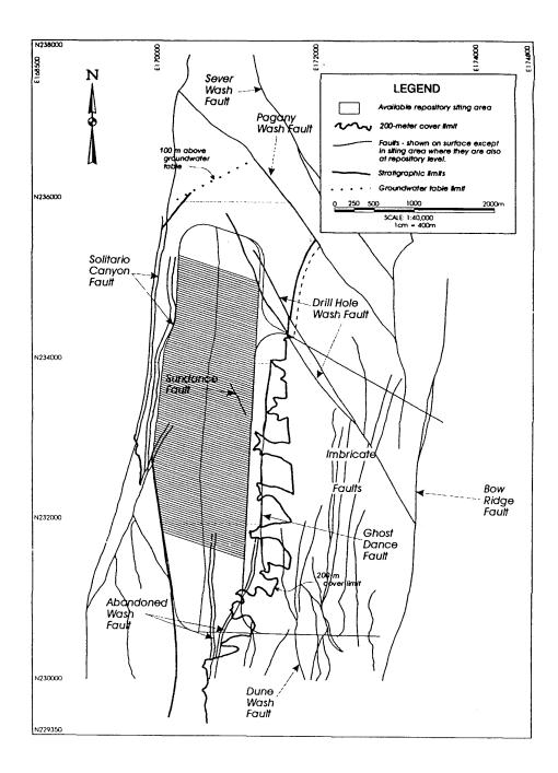
Figure ES.5-2. Repository Layout for the TSPA-VA Design
