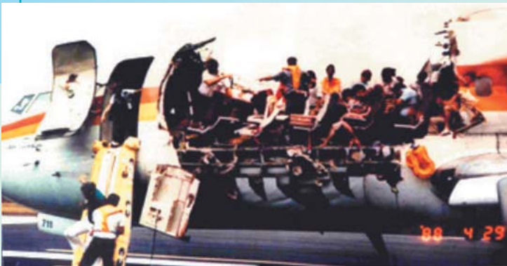
Aloha Airlines Flight 243, near Maui, Hawaii, following the April 1988 accident that was caused by undetected fatigue damage in the 19-year-old aircraft.
