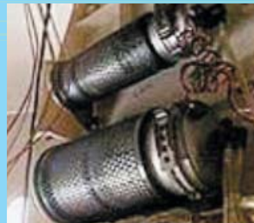
National Transportation Safety Board (NTSB) investigators determined that volatile oxygen-generating canisters stowed in the jet's cargo hold were the cause of the ValuJet airplane crash in the Everglades in 1996.
