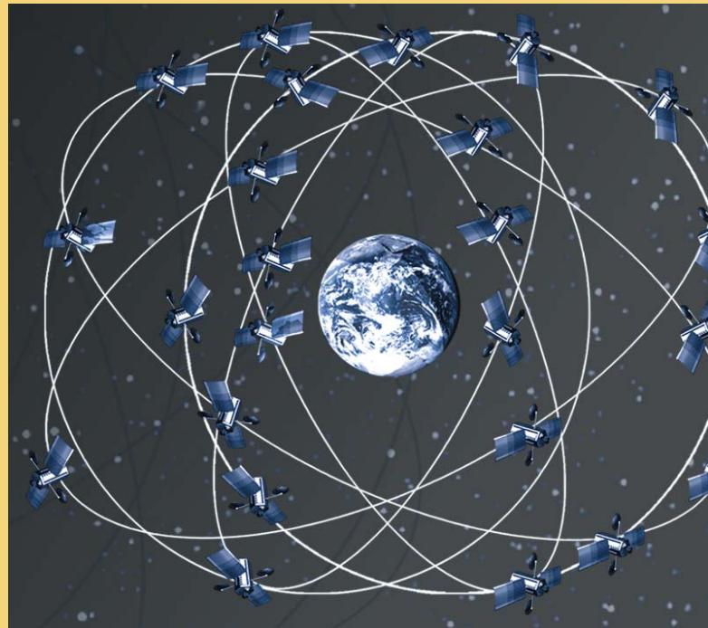
GPS uses a minimum of 24 satellites and ground receivers to track movement for navigation.
