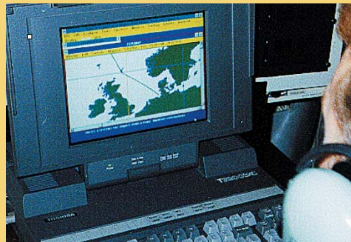
Global information is captured and transmitted every 15 seconds via the INTRANSIT tracking system.
