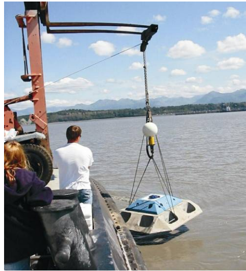
Current meter deployment in Cook Inlet, Alaska
