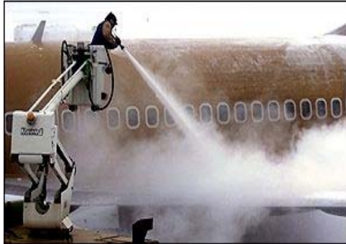
Deicing an aircraft - Unnecessary deicing is a costly proposition for the transportation industry -- photo courtesy BBC
