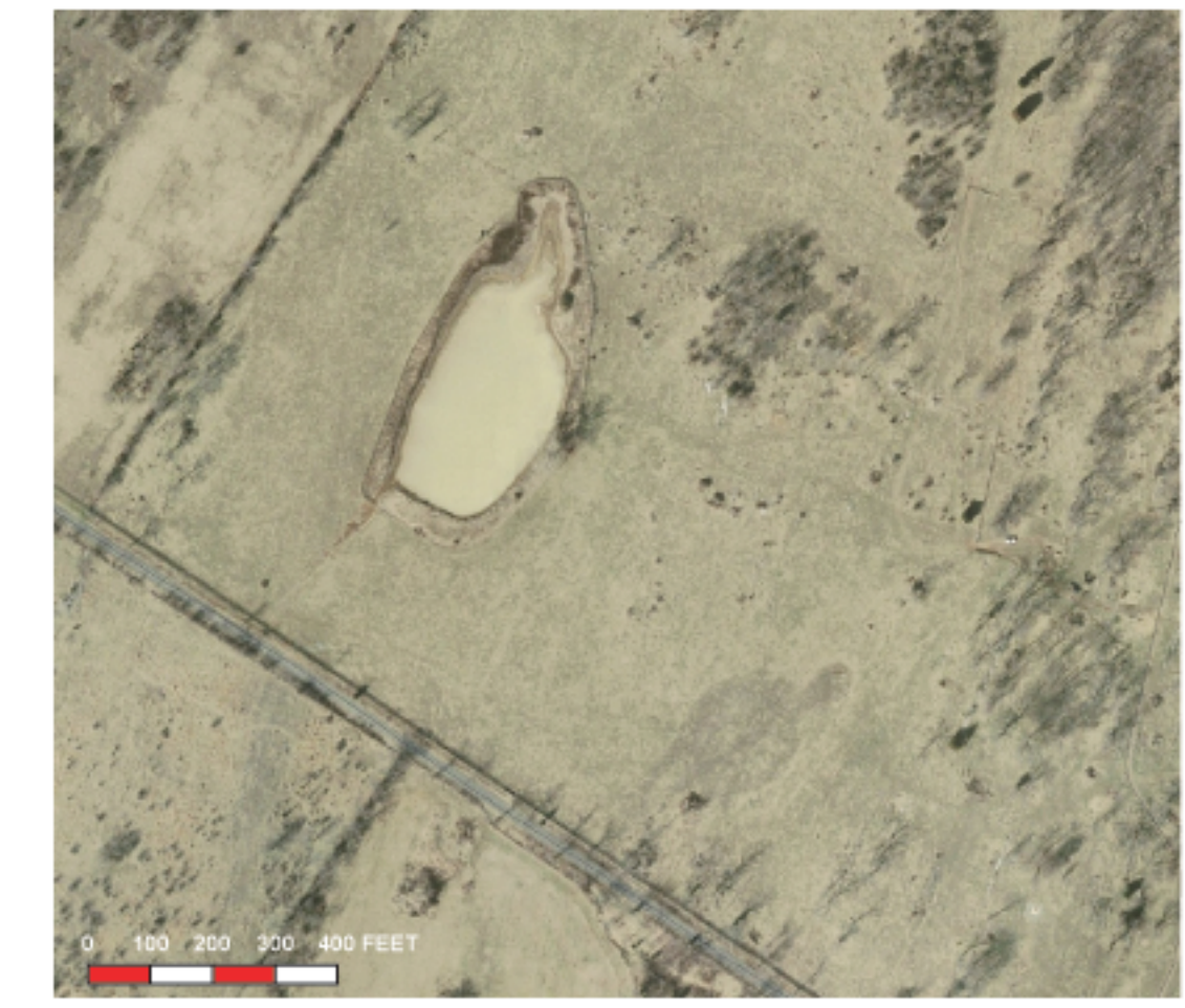
Area along Rt. 620 where ground water overflows along bedding and joints (darker tones) in the carbonate rock in 1996 (wet) and 2002 (drought). Strike of the bedding is to the northeast. North is top of photograph.
