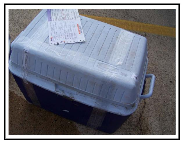
Photo Number: 113 Direction: Down Photographer: Todd Quillen Witness: NA Date: 4/25/07 Time: 1745 Logbook Photo Number: TQ-12 **Description:** Sample cooler ready for shipment from FedEx office in El Dorado, Arkansas, to GPL Laboratory in Frederick, Maryland; note custody seals, taped, and completed FedEx label
