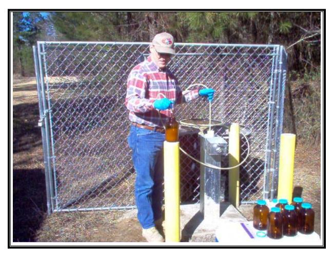
Photo Number: 009 Direction: East Photographer: Tim Osburn Witness: Steve Phillips Date: 02/28/07 Time: 0850 Logbook Photo Number: TO-06 **Description:** View of sampling SW-1 using a waterra valve.
