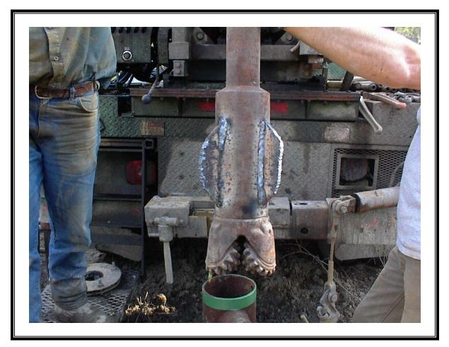
Photo Number: 069 Direction: N/A Photographer: Stephen Phillips Witness: None Date: 3/9/2007 Time: 1542 Logbook Photo Number: SP-29 **Description:** Drill bit used to ream the corehole to an 8-inch diameter
