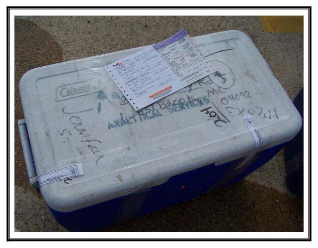
Photo Number: 111 Direction: Down Photographer: Todd Quillen Witness: NA Not available Date: 4/25/07 Time: 1745 Logbook Photo Number: TQ-10 **Description:** Sample cooler ready for shipment from FedEx office in El Dorado, Arkansas, to GPL Laboratory in Frederick, Maryland; note custody seals, taped, and completed FedEx label
