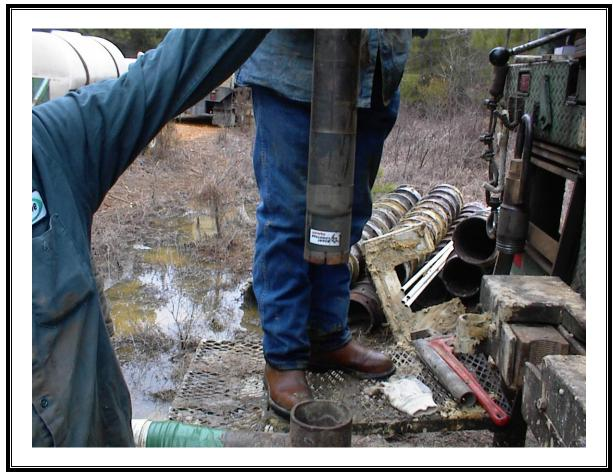
Photo Number: 096 Direction: N/A Photographer: Stephen Phillips Witness: Anna Cornelious Date: 2/8/2007 Time: 1001 Logbook Photo Number: SP-09 **Description:** Core bit on NQ Wireline Barrel used at DW-6.
