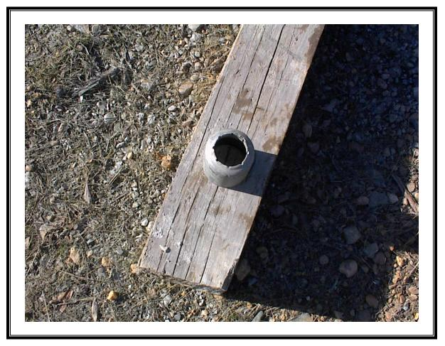
Photo Number: 105 Direction: Down Photographer: Stephen Phillips Witness: None Date: 2/27/2007 Time: 1550 Logbook Photo Number: SP-27 **Description:** Drill bit with diamonds polished off used at DW-7.
