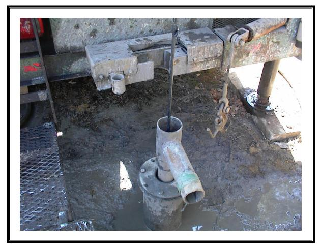
Photo Number: 050 Direction: Down Photographer: Stephen Phillips Witness: None Date: 2/21/2007 Time: 1116 Logbook Photo Number: SP-24 **Description:** Cable attached to probe in DW-3
