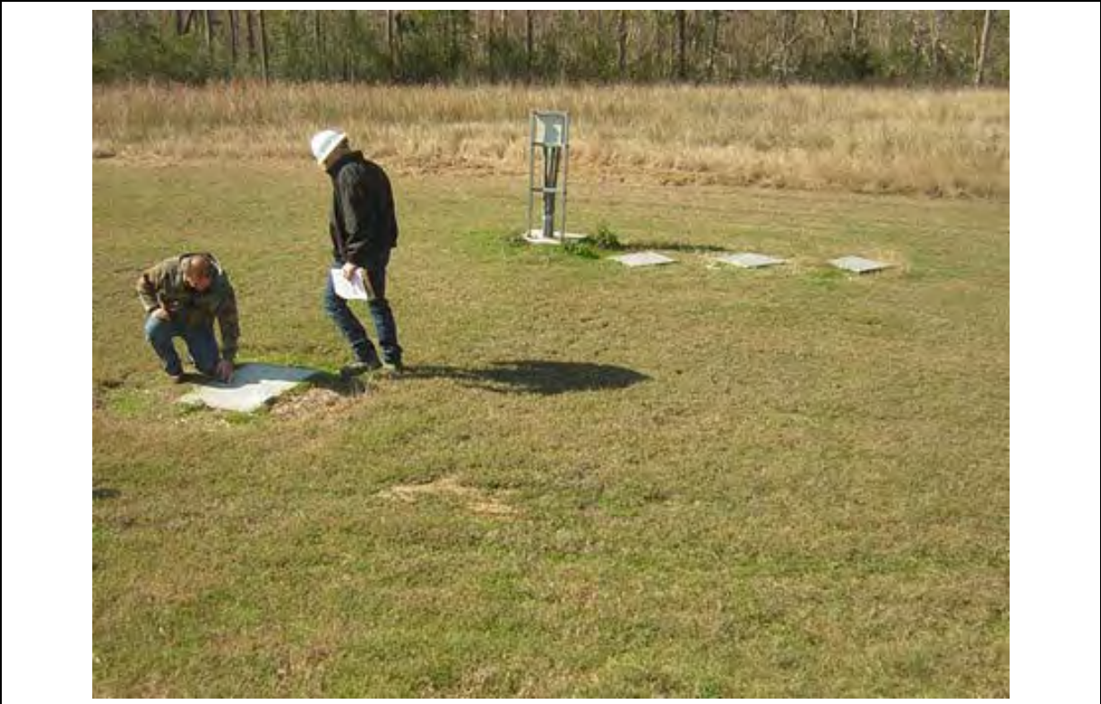
Photo 15: Recovery array 1A well vaults. Taken 2/16/2006
