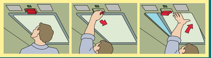
At least one roof hatch, located above the aisle, is also available as an emergency exit. Follow the marked instructions to open the roof hatch.
