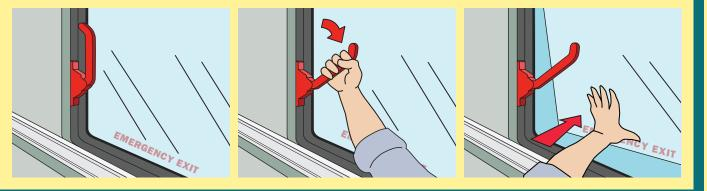
Designated windows are marked as emergency exits and push out to open. Follow the marked instructions to release the lock and open the window.
