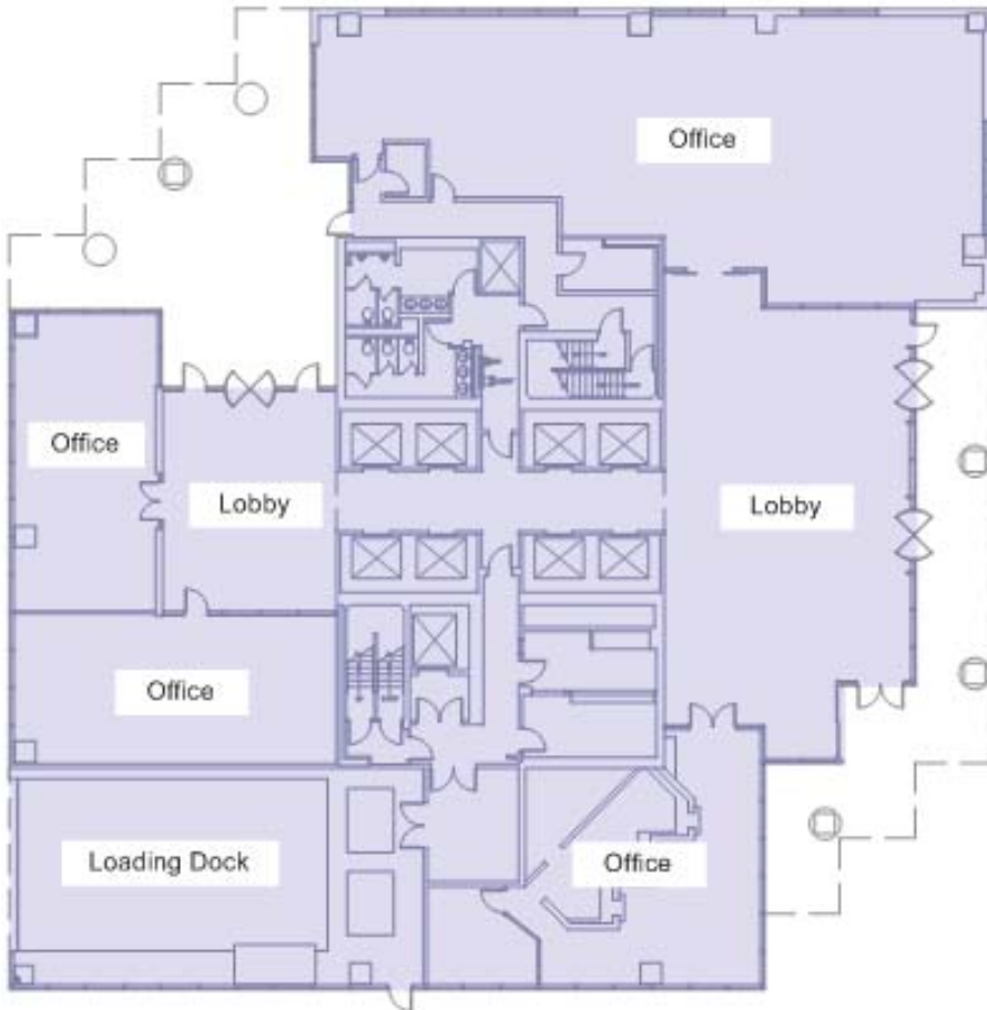
ILLUSTRATION 2.2-1: The shading depicts the Gross of this floor plan. This floor layout depicts required elements that are included in the Gross.
