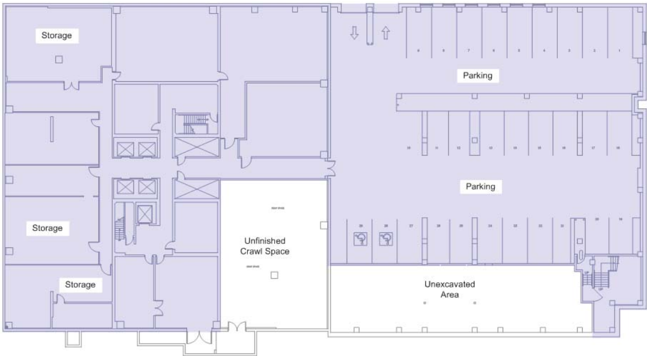
ILLUSTRATION 2.2-2: Basement with unfinished crawl space and unexcavated space. Shading depicts the Gross of this floor plan. Floor plan layout depicts elements for a basement with unfinished crawl space and unexcavated space associated with that level that are excluded from the Gross.
