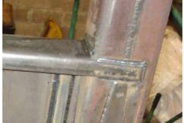
Figure 15. The shelf connection to the corner post, pre-test
