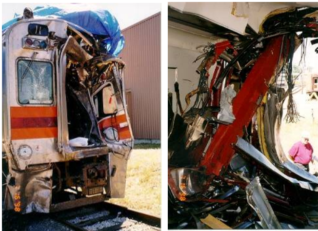
Figure 1. Cab car involved in the grade crossing collision in Portage, Indiana
