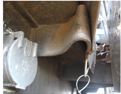
Figure 28. Deformation in the Trailing Locomotive Skirt
