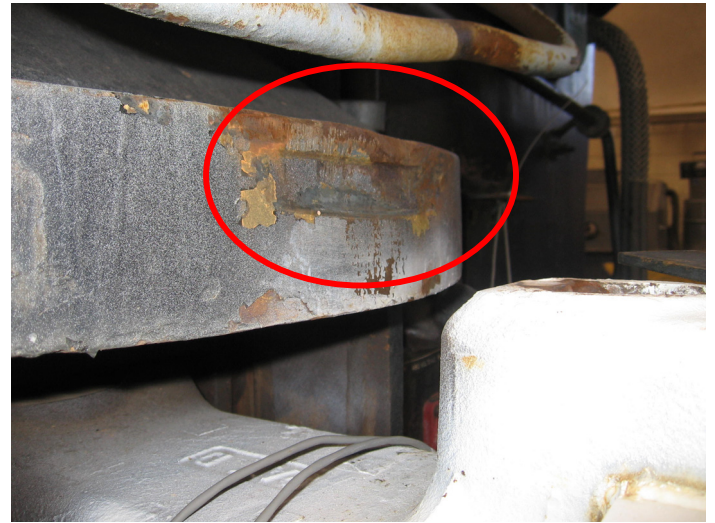
Figure 21. The Locomotive Edge Where It Hit the Anti-Climber
