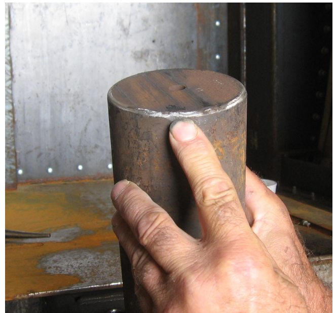
Figure 4. Indentation on Coupler Pin
