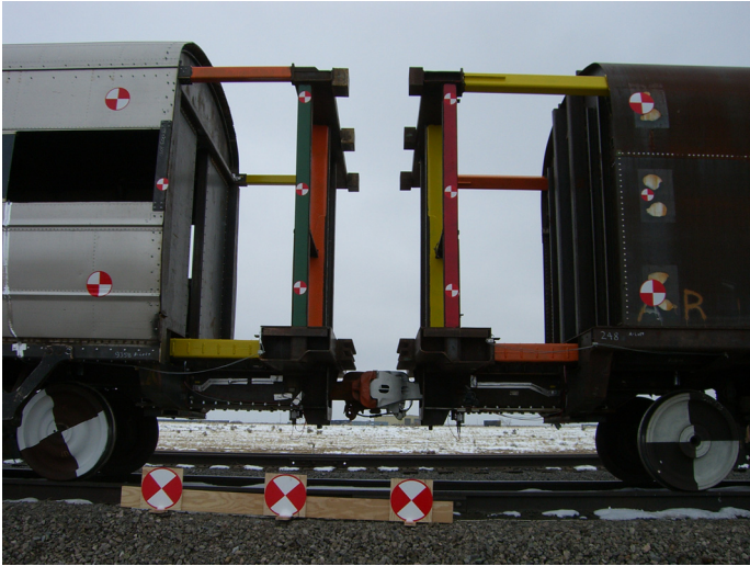
Figure 12. Coupled Interface Pre-Test
