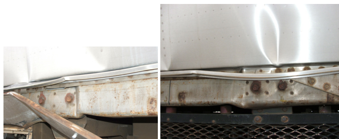
Figure 17. Closeup View of Side Sill Buckle
