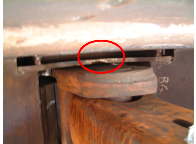
Figure 3. Plate Indented by the Coupler Pin
