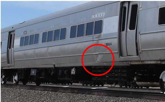
Figure 16. Side Sill Buckle in Budd M1 Car 9614
