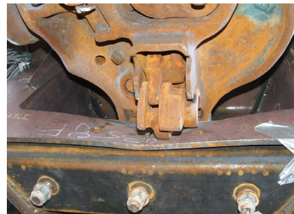
Figure 15. Interaction of the Coupler Lifting Link with the Coupler Carrier
