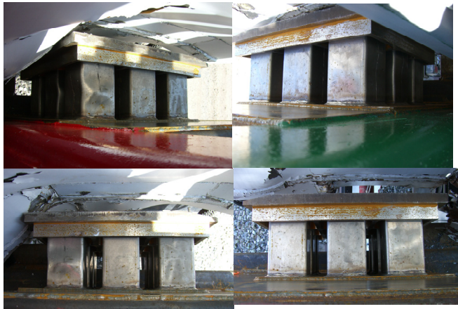
Figure 27. Two Deformable Anti-Climbers from Various Angles
