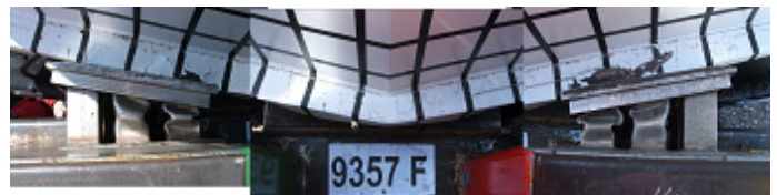
Figure 8. Bird's Eye View of the Deformable Anti-Climbers and the Impacting Locomotive, Post-Test
