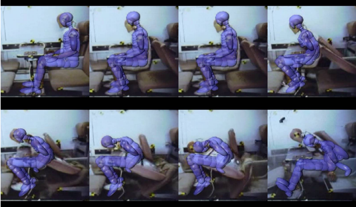
Figure 9. Kinematics of the THOR response in the post-test MADYMO simulation of the CEM two-car full-scale test.
