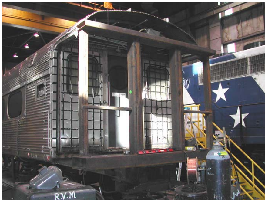
Figure 9. Modified Cab Car End Frame
