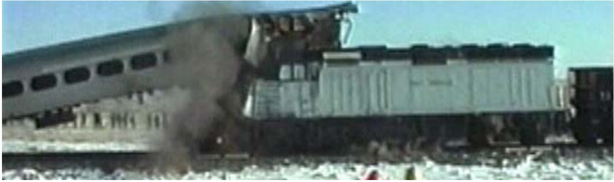
5. Maximum vertical displacement of cab car
