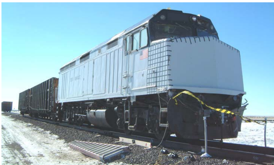
Figure 10. Locomotive-Led Consist from Train-to-Train Test, Prior to Test
