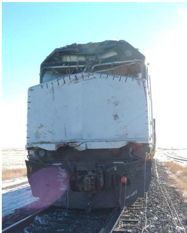
Figure 15. Impacted Locomotive, After Test
