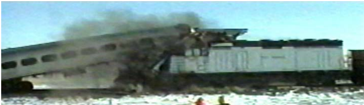
Figure 11. Frame Showing Cab Car at Maximum Override of Locomotive
