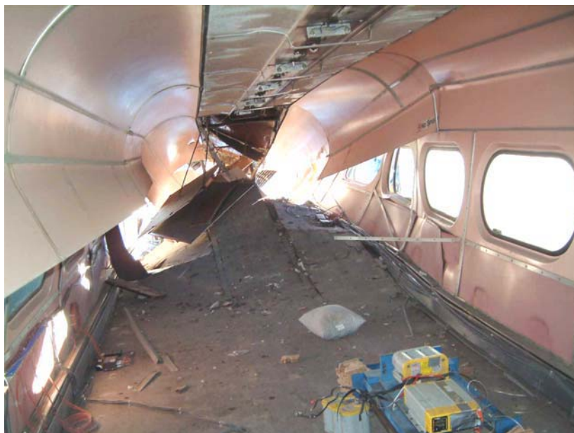
Figure 14. Interior of Cab Car, Looking Toward Crushed End-Led Consist from Train-to-Train Test, After Test
