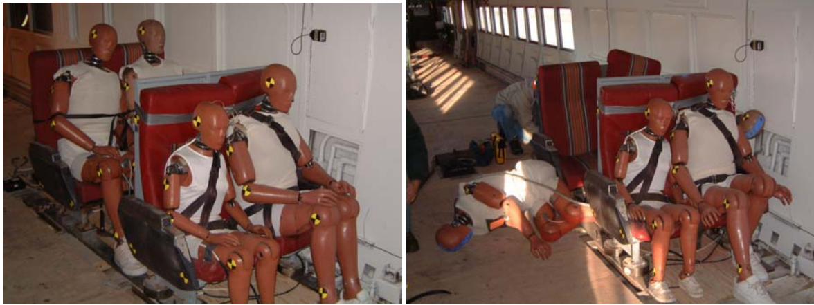
Figure 19. Test Dummies in Inter-City Passenger Seats in Cab Car, Before and After Test
