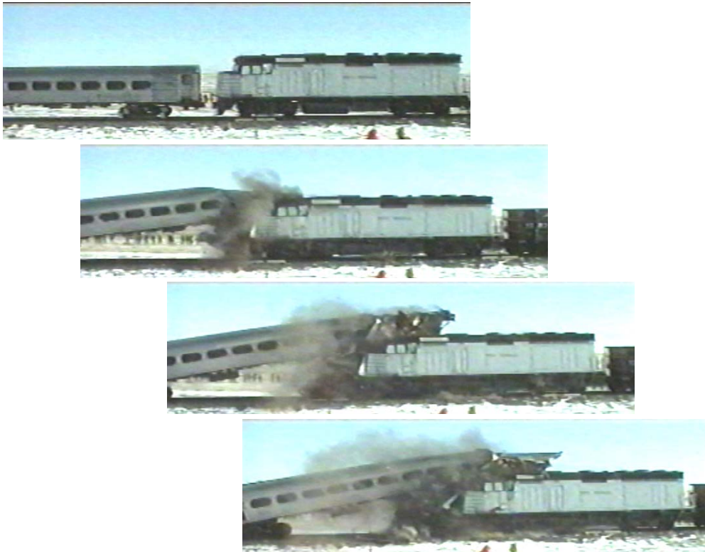
Figure 7. Sequential photos of the in-line train-to-train test
