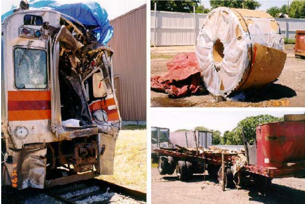
Figure 9. Photos of the steel coil used in the grade crossing test, and the crush of the cab car after the collision
