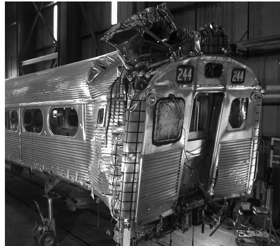
Figure 3. Front and Right Side Car Body Crash Deformations
