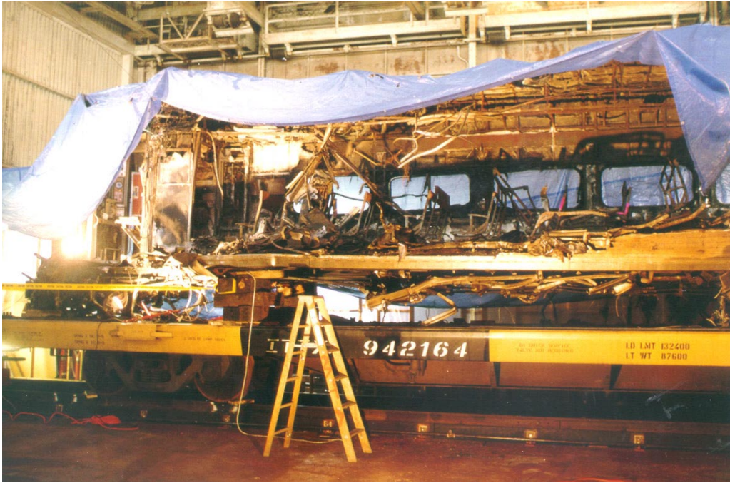
Figure 17. Post-accident photograph, lead cab car, commuter train, Silver Spring, Maryland collision.
