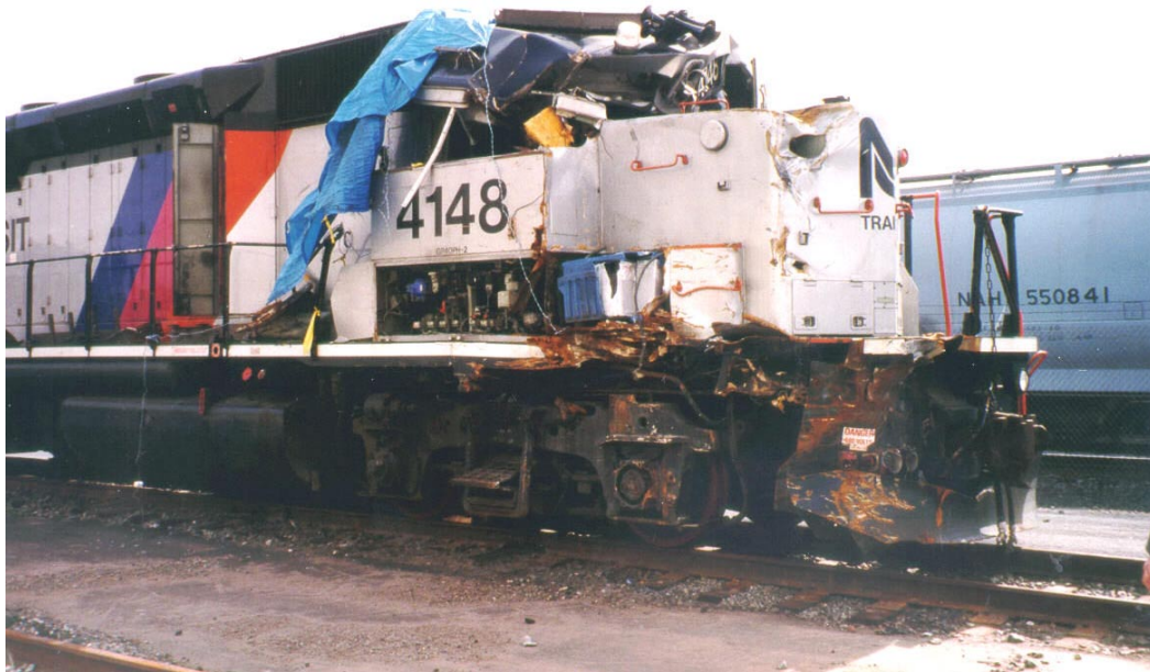
Figure 12. Post-accident photograph, impacted locomotive, Secaucus, New Jersey collision.
