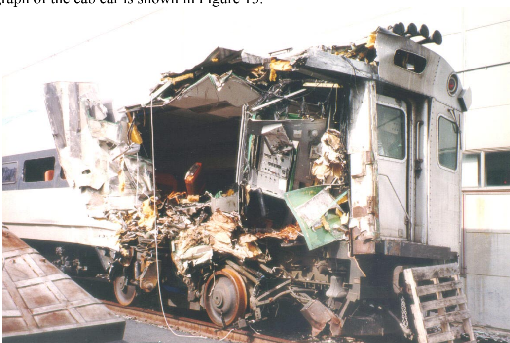
Figure 13. Post-accident photograph, lead cab car, Secaucus, New Jersey collision.
