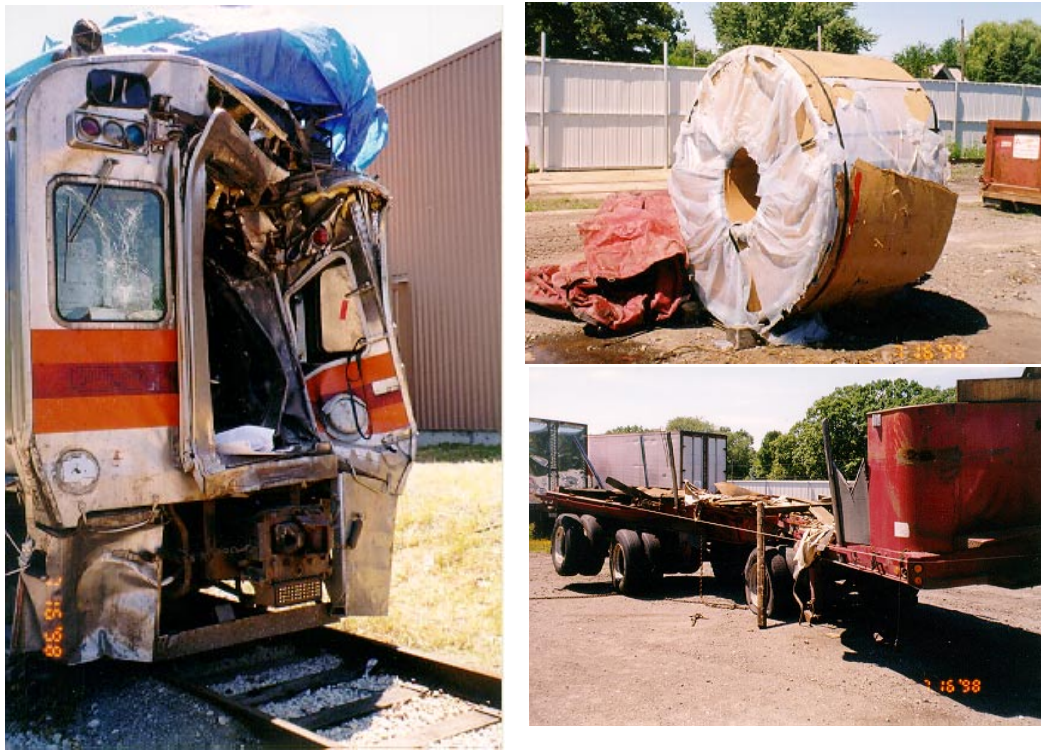
Figure 20. Post-collision photographs, cab car, truck trailer, and steel coil involved in Portage, Indiana grade crossing collision.
