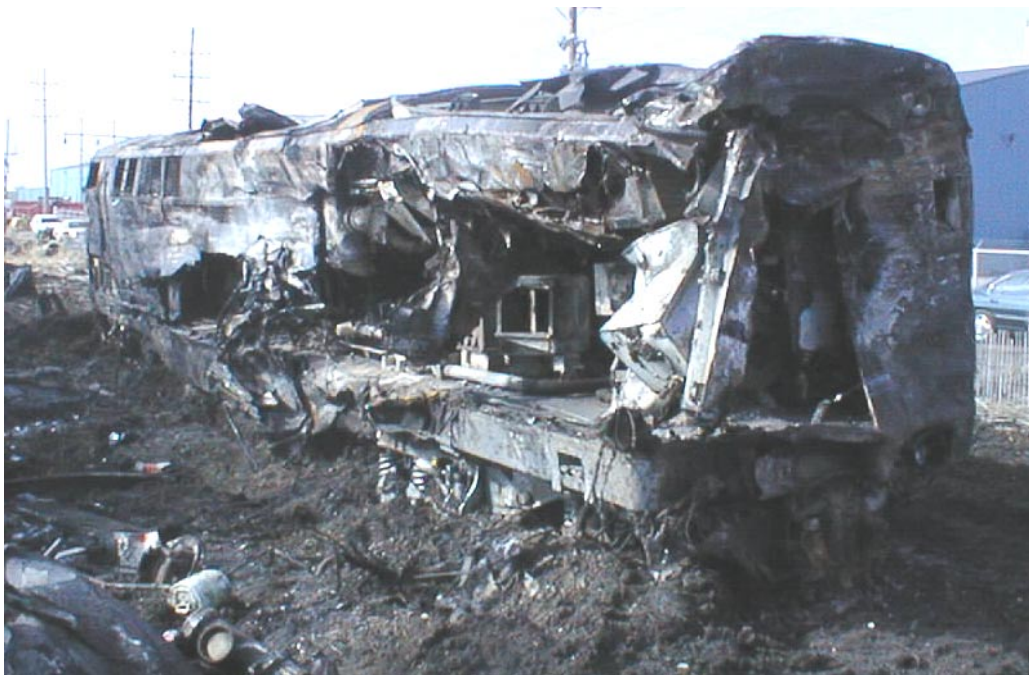
Figure 8. Post-Accident Photograph, Lead Locomotive, Bourbonnais, Illinois Collision.
