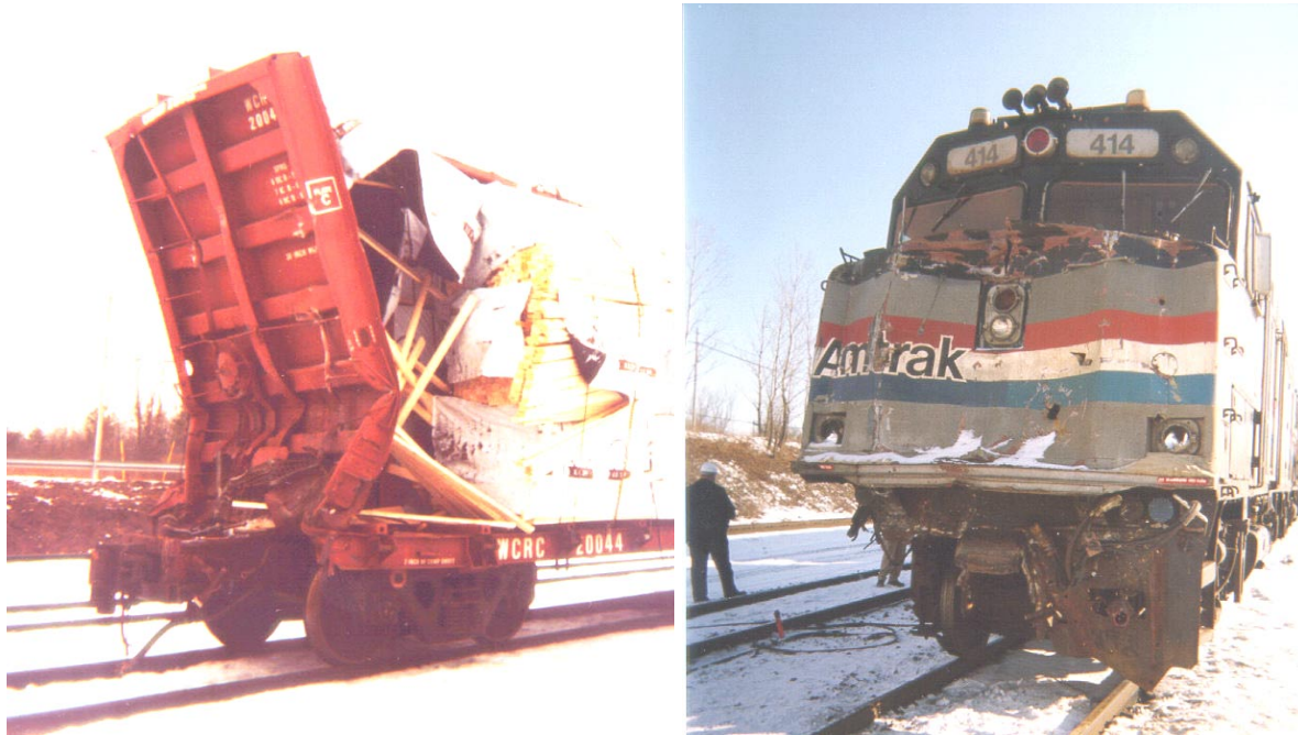
Figure 6. Post-accident photographs, passenger train lead locomotive and freight train trailing loaded bulkhead flatcar, Syracuse, New York collision.
