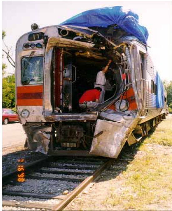
Figure 3. The front end of the cab car following the collision.
