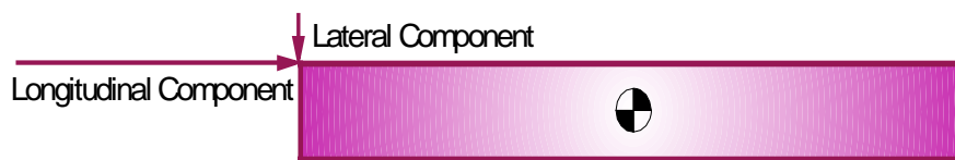
Figure 2. Schematic drawing of minimum lateral force component required to deflect a long slender body, drawn approximately to scale.
