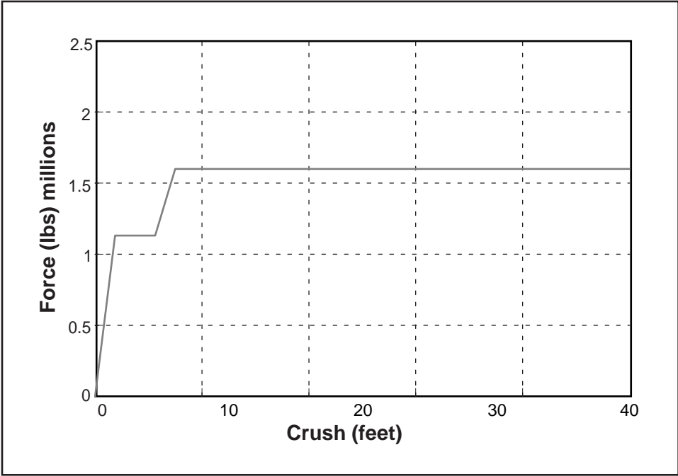
Figure 2-10. Commuter MU Train Car-to-Car Crush Characteristic
