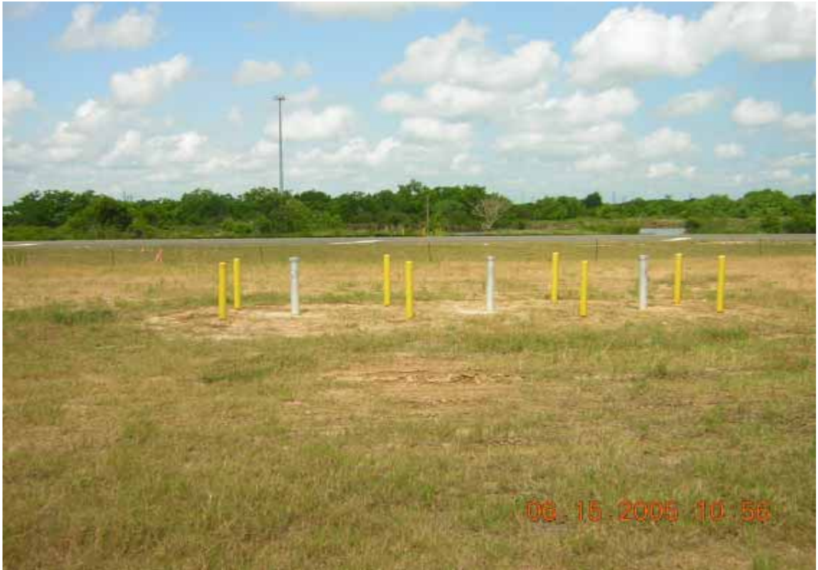
Photo 9: OU1: Site groundwater monitoring wells. ID tags and locks are in place.
