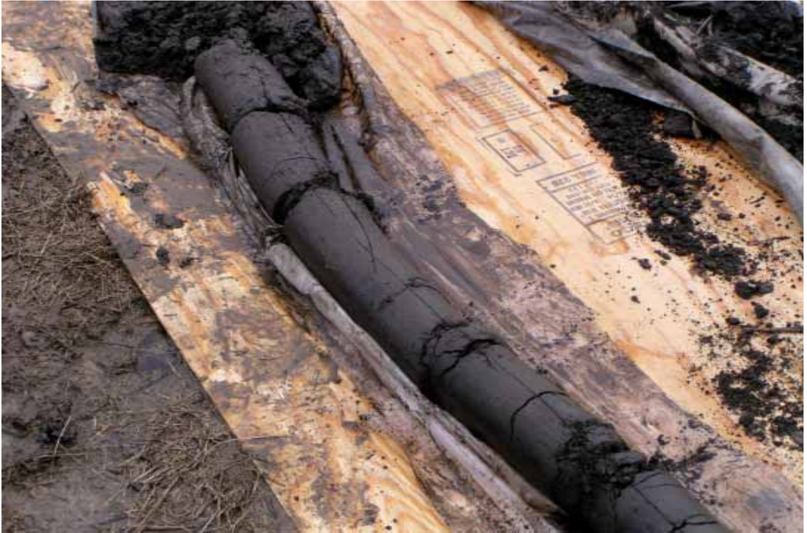
The extruded core was placed on a plywood board for sampling. The cores were collected from the upper 6 feet of treated waste material.
