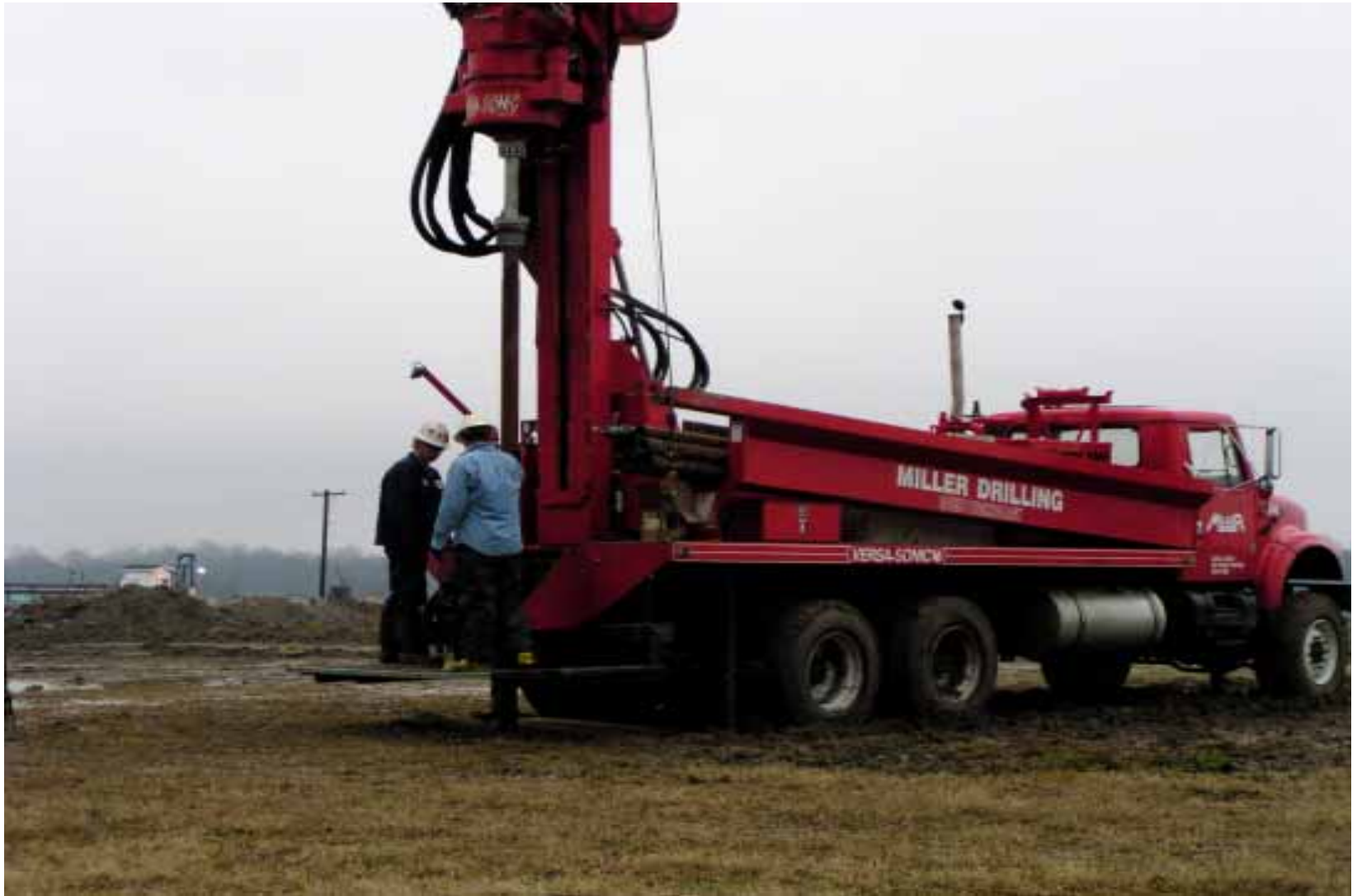
The rotasonic drilling method was used to collect cores from the treated oily sludge pit mound area. The locations were selected in the northern half of the mound area where the sludge was stabilized/solidified using an in-situ auger. The view is toward the northeast with the northernmost barge terminal in the background.
