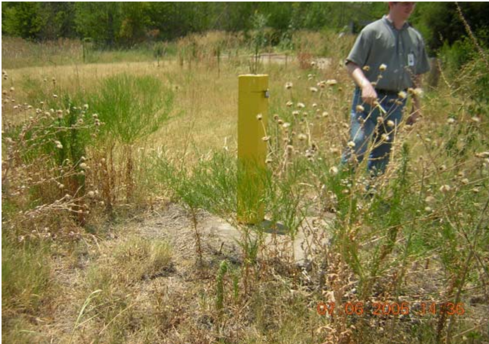
Photo 29: OU5, Subarea 1 – View of a monitor well at the site, located near the former UST area.
