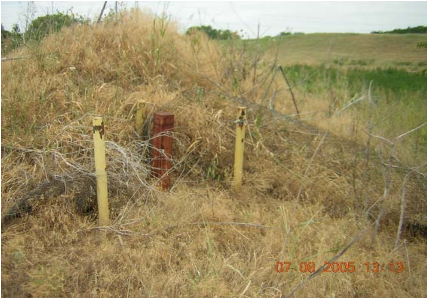
Photo 26: OU3, Site 4 – View of monitor well at site. The well is almost covered by vegetation.
