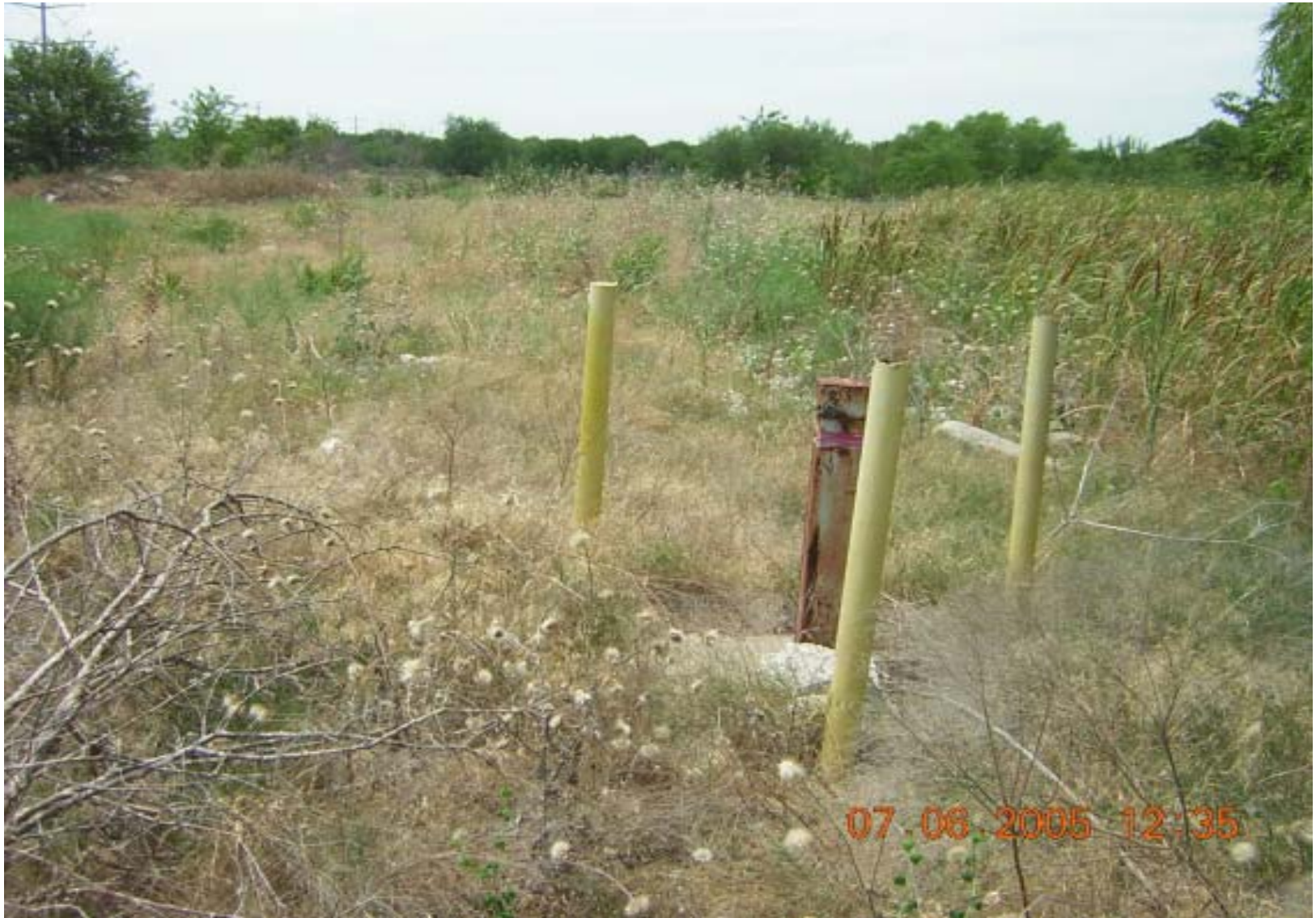
Photo 20: OU3, Site 3 – View of a monitor well installed at the north end of the site.
