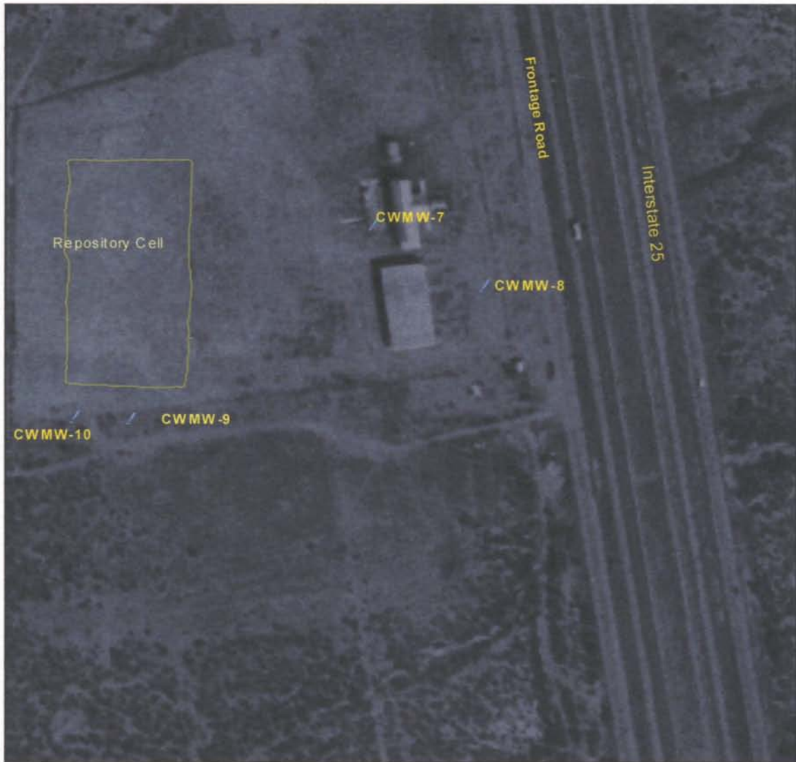
Figure 3: Cal West Metals Repository and Monitoring Well Location
