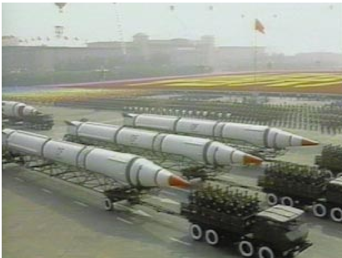
The CSS-2 , manufactured in the early 1960s, was among the PRC's first ballistic missiles. It showed strong Soviet design influences, especially in the guidance and propulsion subsystems.
