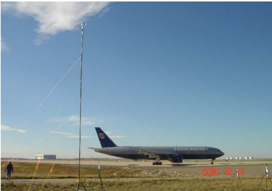
Figure 7. Picture Showing 1.8 and 10 Meter Sonic Anemometer and PM 2.5 Samplers (Note: Aircraft shown is in a holding area and was too close for effective LIDAR sampling.)
