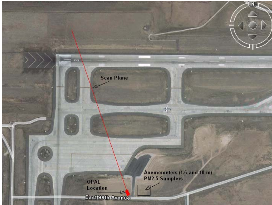
Figure 4. OPAL Location in Relation to Runway 08 and Scan Plane (Ambient PM2.5 and anemometer general area also shown)
