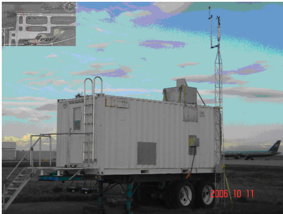
Figure 5. OPAL System Showing Aircraft on Near Taxiway (Runway 08/26 in Far Background)
